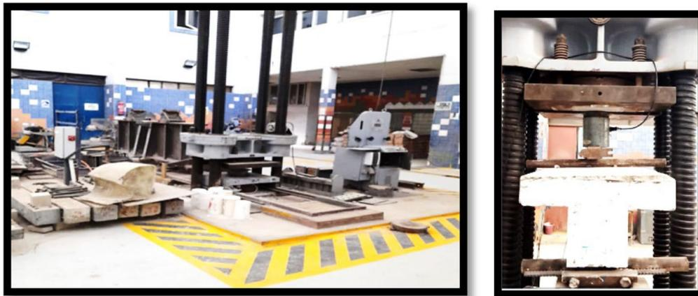
**Fig.10** Hydraulic jack (5000 K N) on the loading plates
