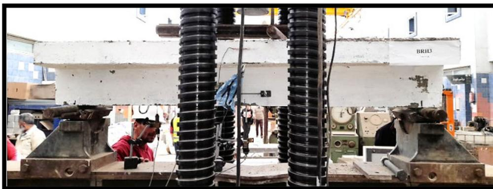
**Fig.9** The test loading of the specimens, LVDT and strain gages for specimens
