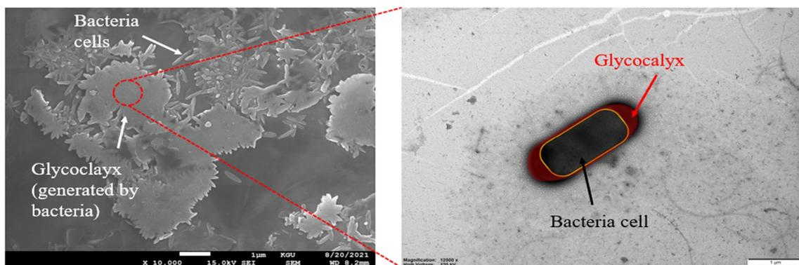
**Fig. 4** Typical SEM and TEM images for bacterial colonies and glycocalyx immobilized in porous of expanded vermiculites
