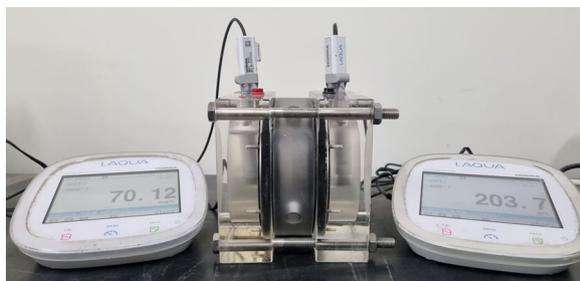
Fig. 5 Typical setting images of natural diffusion cell test
