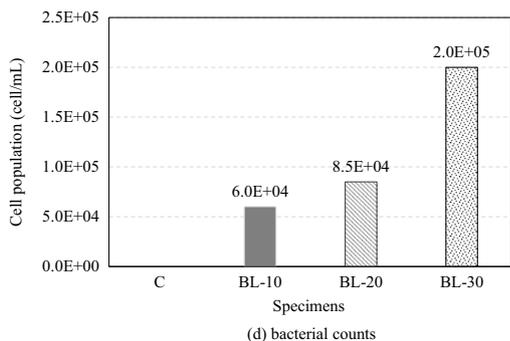
Fig. 9 Bacterial colonies and cell population counts results from the hardened mortars exposed to NaCl solutions for 91 days
