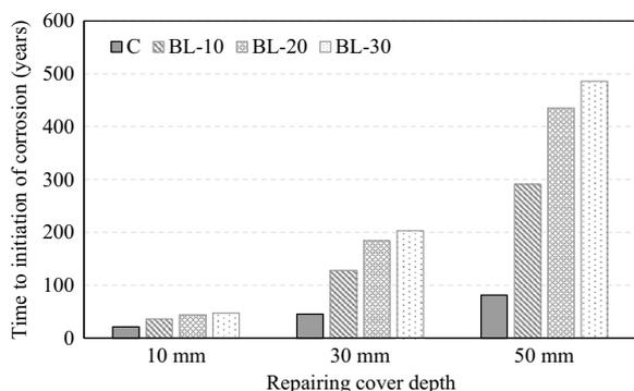
**Fig. 11** Expected service life of concrete structures repaired using mortar specimens at different thicknesses
