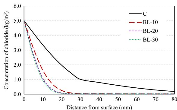
Fig. 10 Analytical chloride ion concentration profiles in the concrete structures repaired using mortar specimens at a thickness of 30 mm
