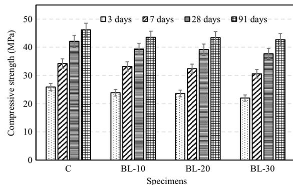
Fig. 6 Compressive strength of specimens at different ages
