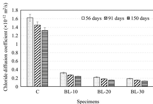
**Fig. 7** Chloride diffusion coefficient of specimens at different ages
