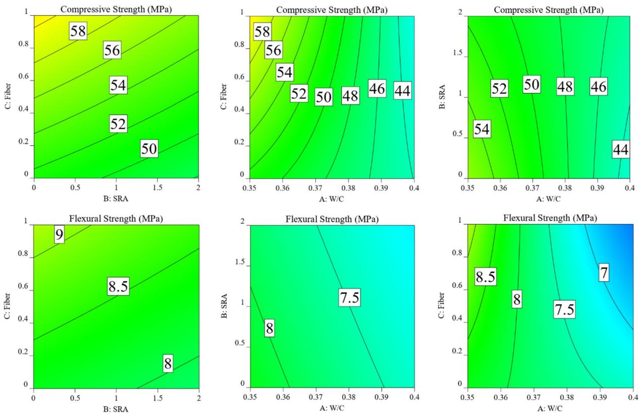
**Fig. 2** RSM plots for compressive (top) and flexural (bottom) strength results
