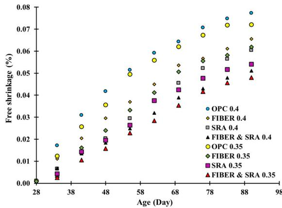
**Fig. 4** Results of free shrinkage of all concrete mixtures
