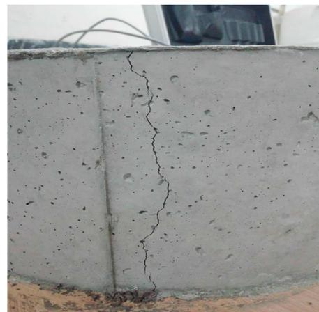
**Fig. 7** Image of OPC specimen at the age of 60 days for evaluating crack width
