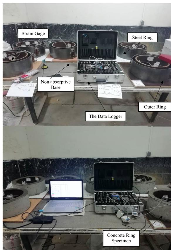
**Fig. 1** Specimen mold before the test (Top) and molded concrete specimen under data acquisition (Bottom)
