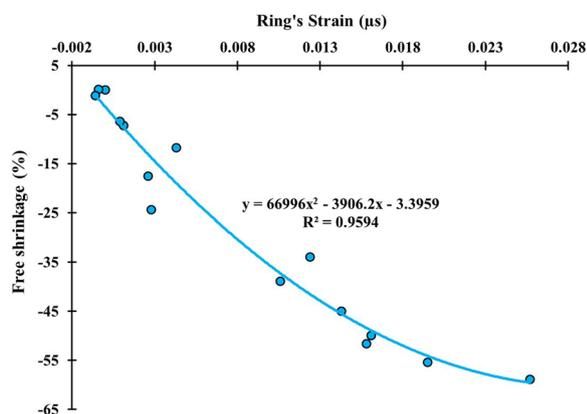
**Fig. 8** The relationship between the results of free and restrained shrinkage
