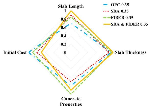
**Fig. 9** The effect of using SRA and polypropylene fiber on concrete pavement properties
