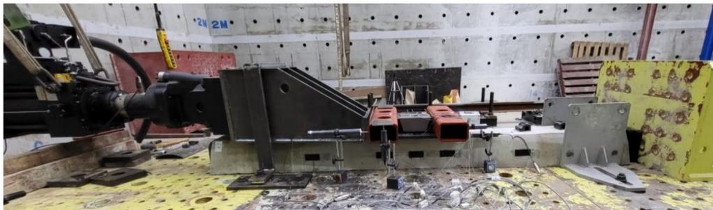
**Fig. 6** Loading set-up for element-level specimens
