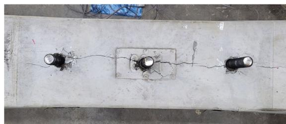
**Fig. 9** Damage for element level specimen S\_DCP-2
