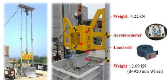
**Fig. 3** Drop weight test (Kim et al., 2019, 2020)
