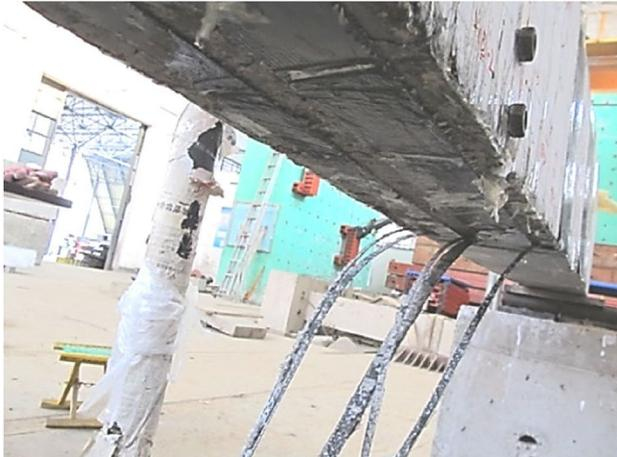
**Fig. 4** Failure mode of RAC beams strengthened by one layer CFRP
