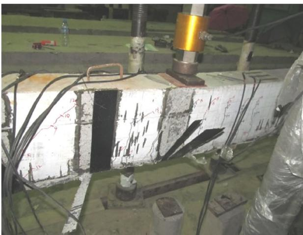
**Fig. 5** Failure mode of RAC beams strengthened by two layers CFRP
