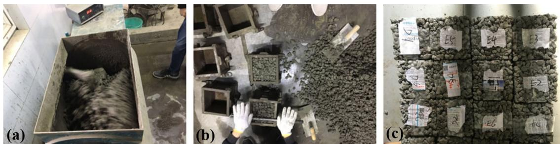
**Fig. 3** Specimen preparations. **a** Concrete mixing; **b** concrete molds; **c** samples number
