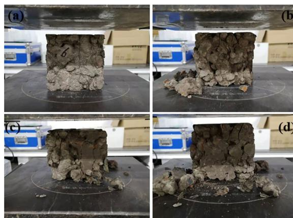
**Fig. 7** Failure characteristics of five groups, including a–c aggregate failure and d ITZ failure
