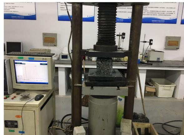
**Fig. 5** Test setup of compressive strength for the PCs
