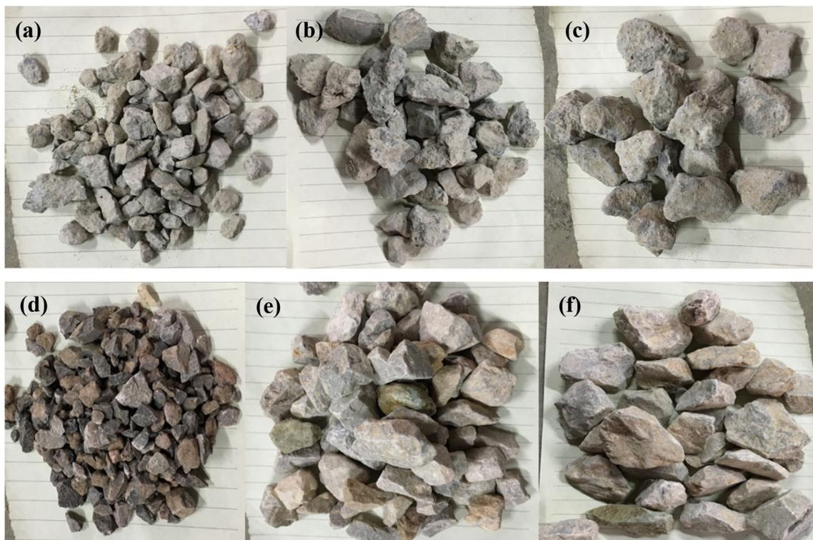
**Fig. 1** Recycled coarse (a 4.75–9.5 mm, b 9.5–19 mm and c 19–31.5 mm) and Natural aggregates (d 4.75–9.5 mm, e 9.5–19 mm and f 19–31.5 mm) particle size ranges used
