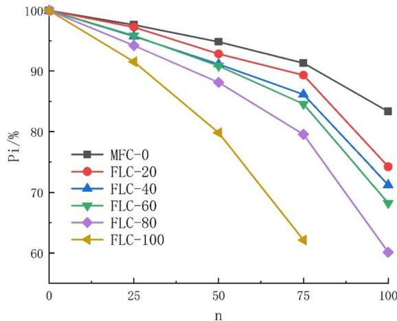
**Fig. 3** The relationship curve between the relative dynamic elastic modulus of MFC and the number of freeze-thaw cycles
