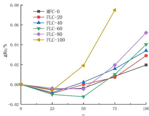
**Fig. 2** The relationship curve between the mass loss rate of MFC and the number of freeze–thaw cycles
