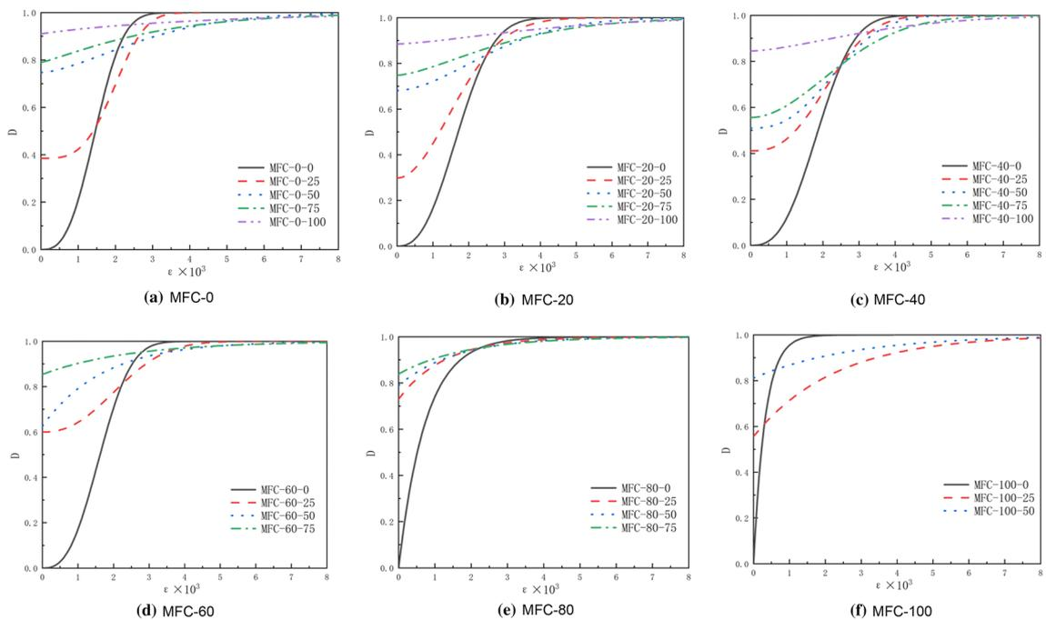
**Fig. 8** Relationship between total damage variable  $D$  and strain under different times of freeze–thaw cycles
