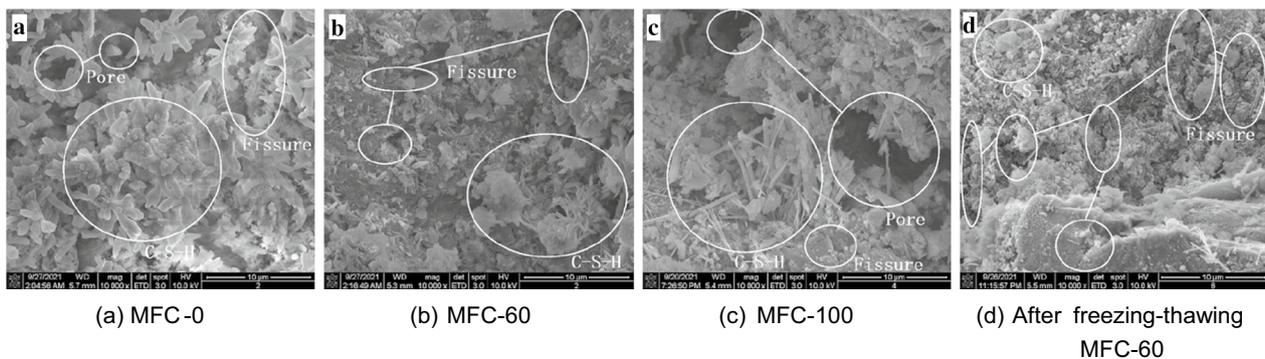
**Fig. 5** SEM comparison diagram. The figure (a, b, c) show the SEM images at different substitution rates before the freeze–thaw cycles
