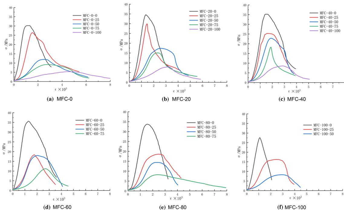
**Fig. 4** The stress-strain full curve of different freeze-thaw cycles of MFC concrete
