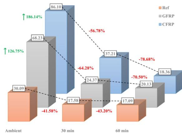
**Fig. 14** Changes in compressive strength of the non-insulated specimens
