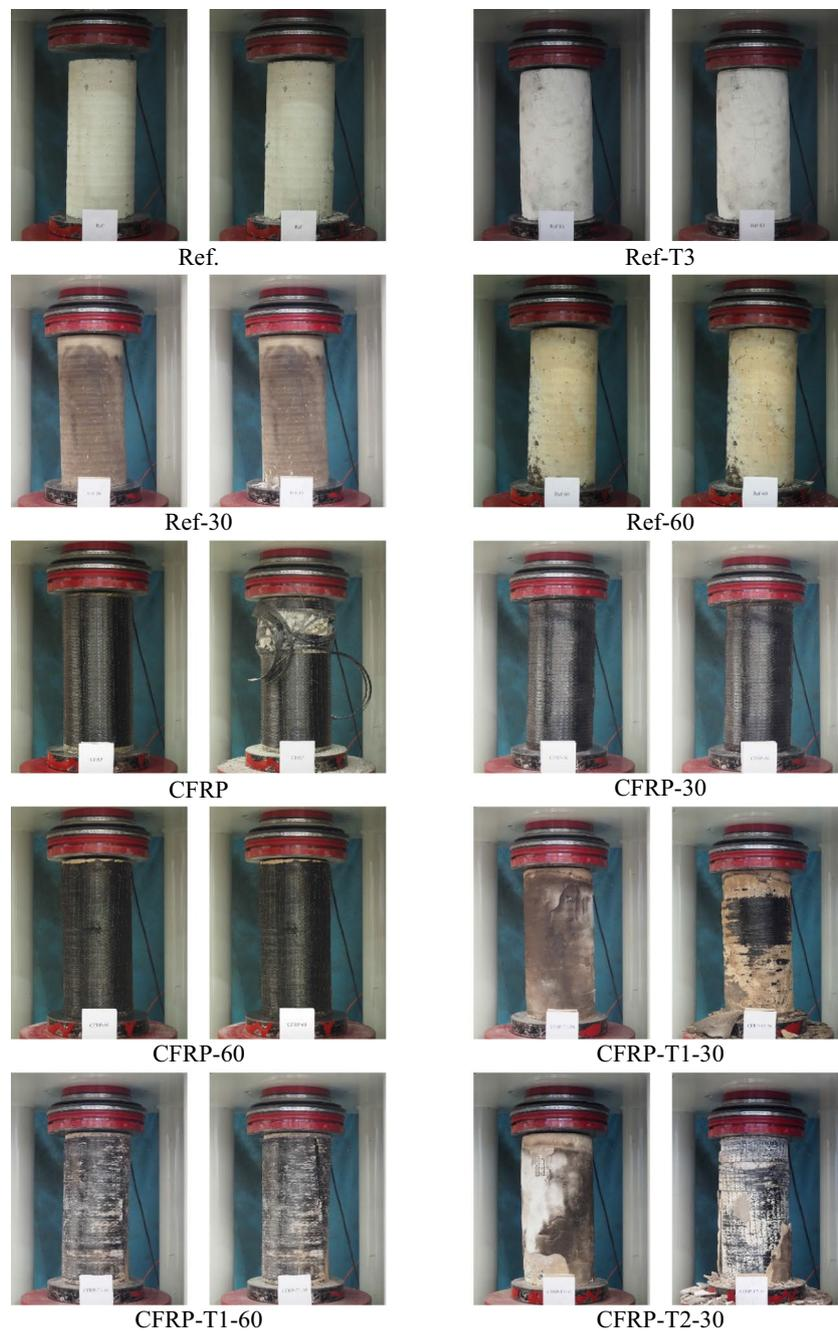
**Fig. 11** Testing compressive strength of REALROCK samples before and after the fire tests
