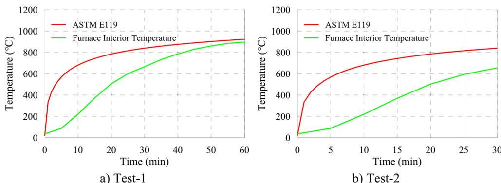
**Fig. 7** ASTM E119 fire curve and furnace interior temperatures during the tests
