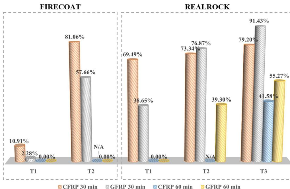
**Fig. 17** The success of insulation systems in maintaining the strength provided by FRP
