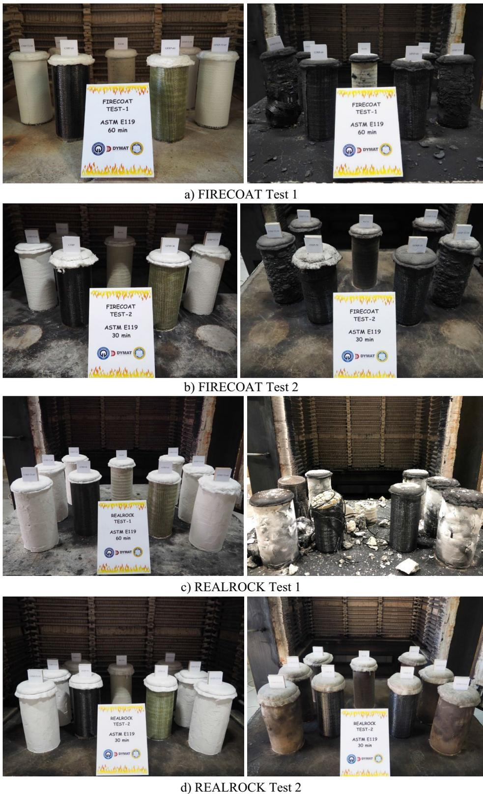
**Fig. 9** Pre and post-test conditions of the specimens
