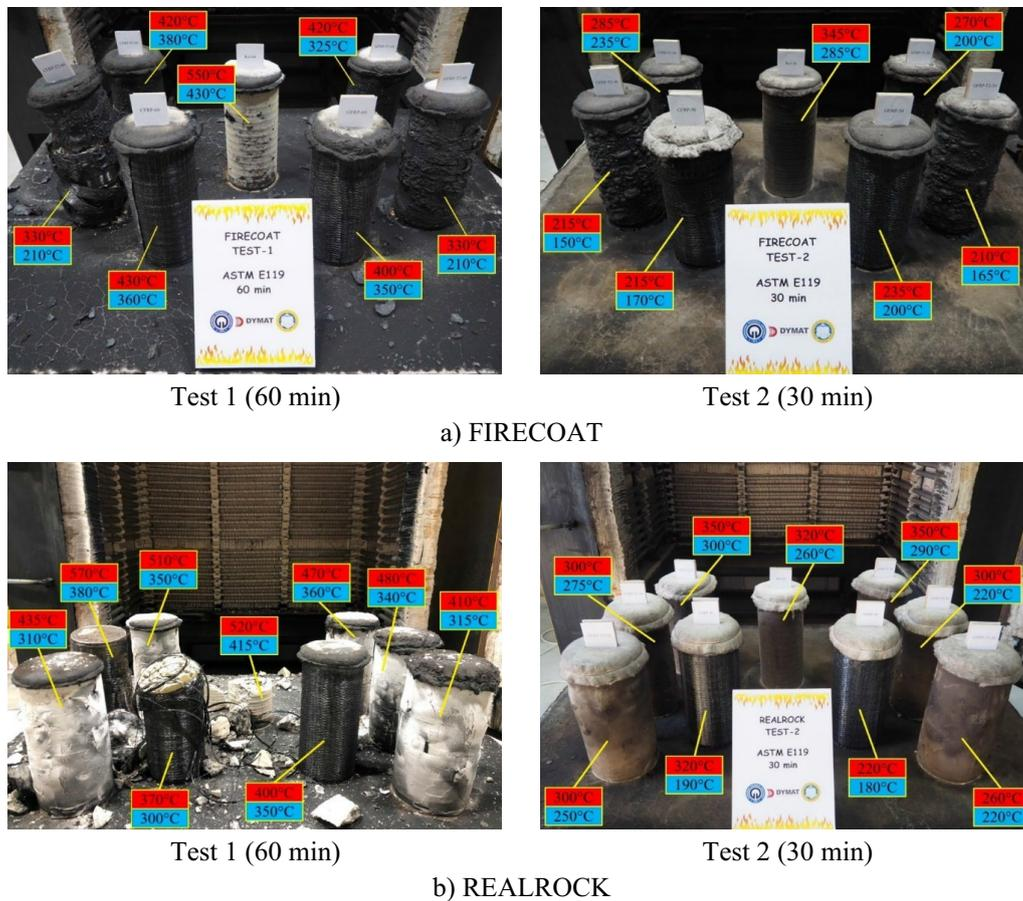
**Fig. 12** Measured values of surface temperatures
