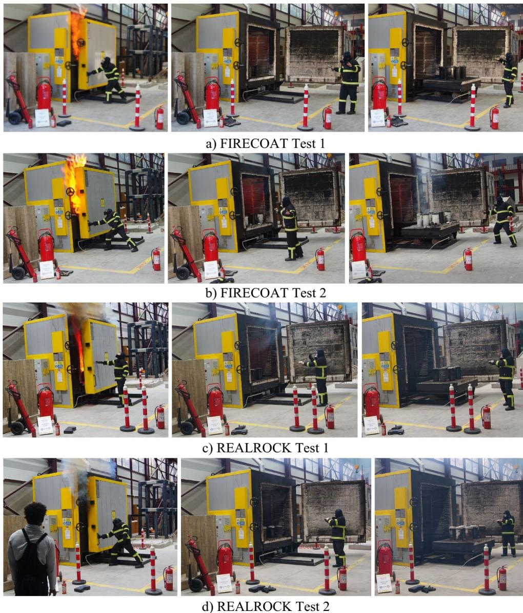
**Fig. 8** Opening furnace door and surface temperature measurements
