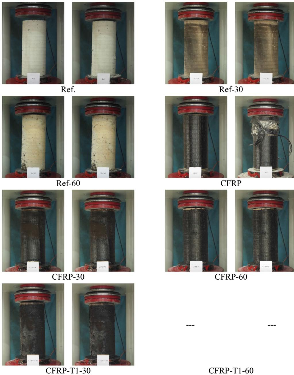
**Fig. 10** Testing compressive strength of FIRECOAT samples before and after the fire tests
