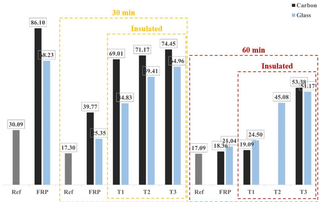
Fig. 16 Compressive strength of the tested specimens for REALROCK
