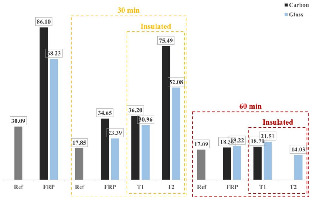
Fig. 15 Compressive strength of the tested specimens for FIRECOAT
