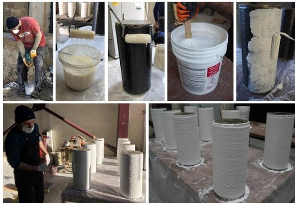
**Fig. 3** Preparation and application of the FIRECOAT components
