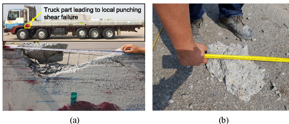
Fig. 8 (a) Punching shear failure at top of the CMB-17S and (b) concrete fragmentation from the CMB-17S caused by punching shear failure
