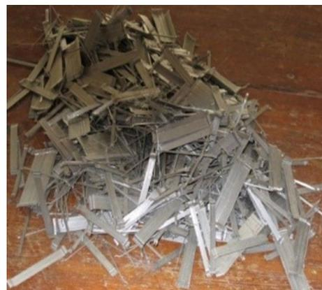
**Fig. 1** Steel fiber.
