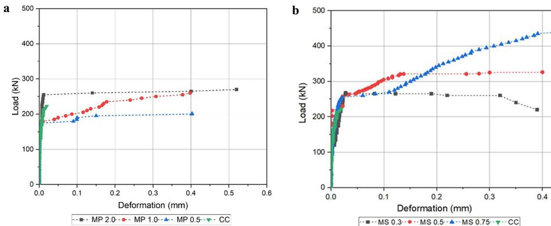
Fig. 10 a Effect of polyester fibers on split toughness of single FRC system. b Effect of steel fibers on split toughness of single FRC system.
