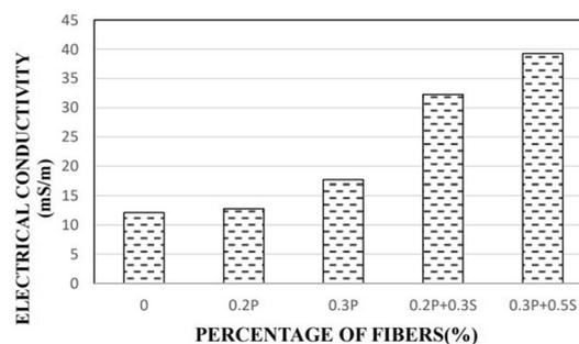
**Fig. 13** Electrical conductivity of FRC with various fiber content.
