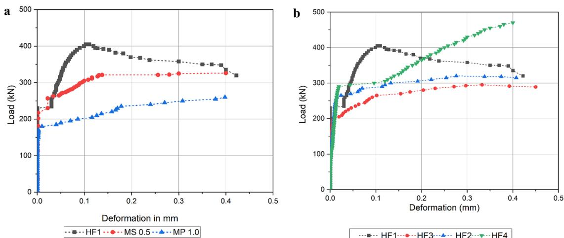
**Fig. 11** a Load–deformation curve of single and hybrid FRC. b Load–deformation curve of hybrid FRC.
