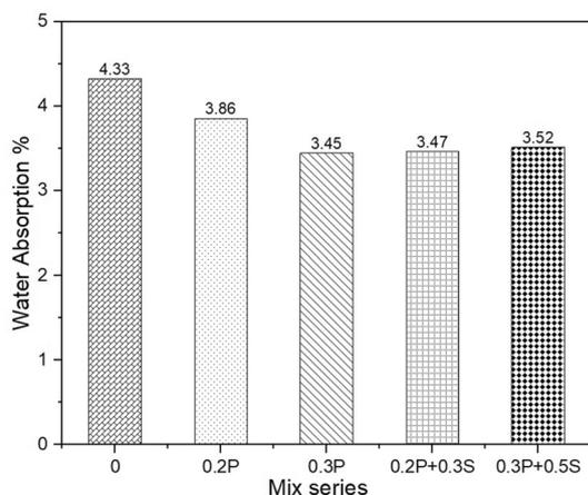
**Fig. 12** Water absorption of FRC with various fiber content.
