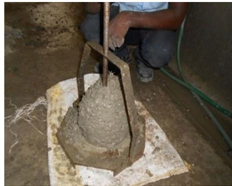
**Fig. 3** Slump test.
