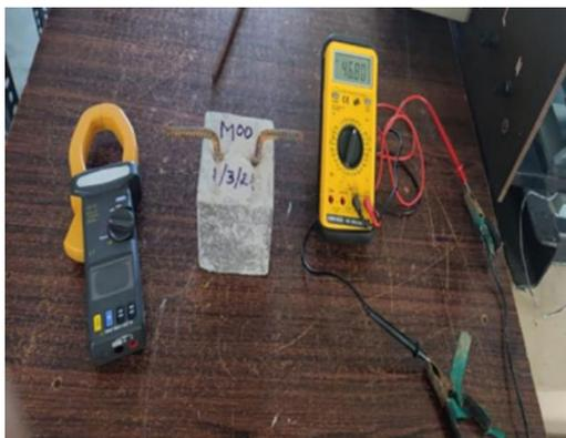
**Fig. 7** Bulk electrical conductivity test.
