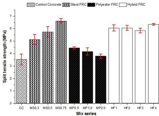
Fig. 9 Split tensile strength.
