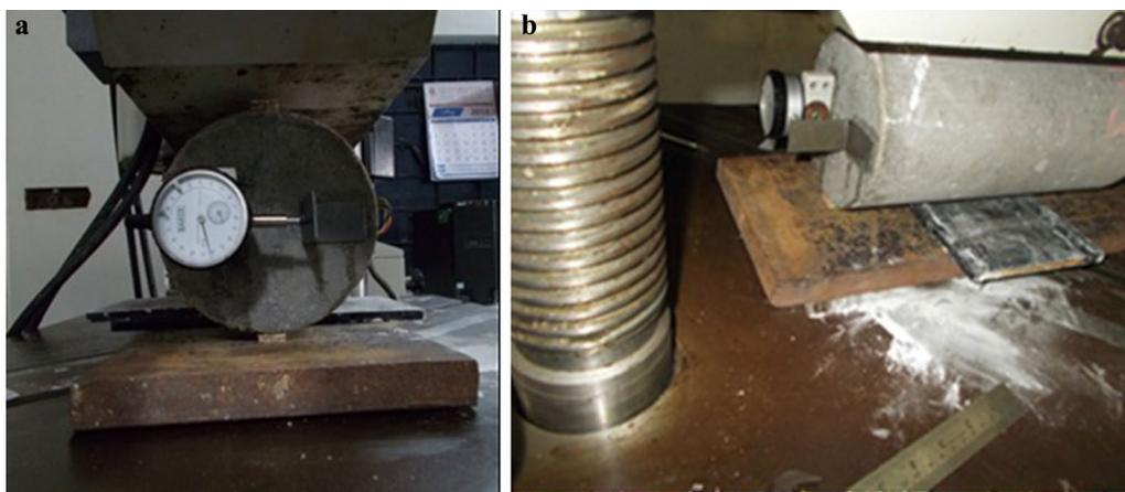
**Fig. 4** **a** Testing arrangement of split tensile toughness. **b** Testing arrangement of split tensile toughness.
