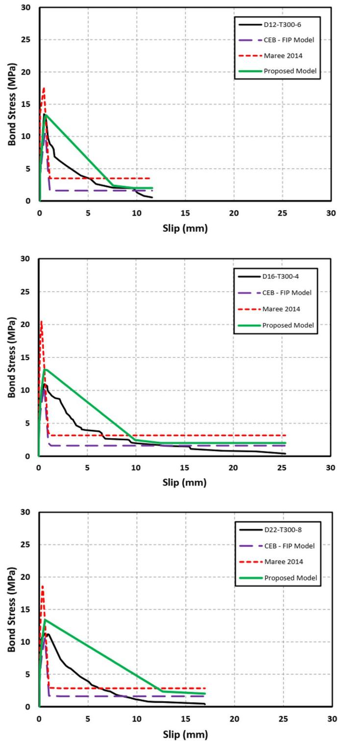
**Fig. 24** Proposed analytical versus experimental bond–slip relationships (elevated temperature of 300 °C)
