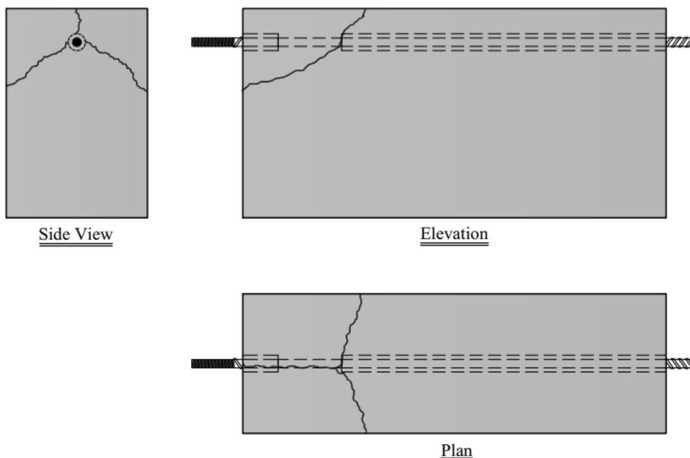
**Fig. 12** Typical cracking pattern of the tested beam-end specimens
