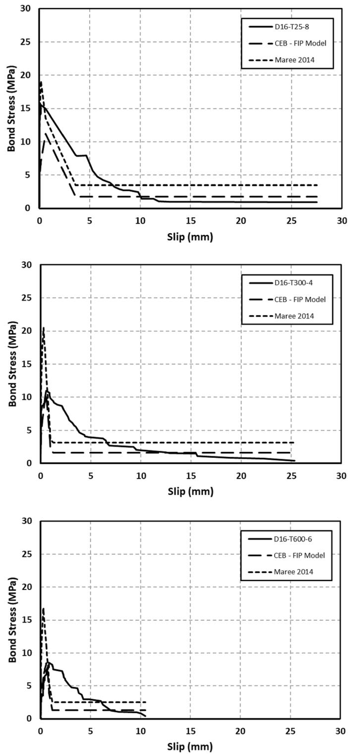
**Fig. 21** Analytical versus experimental bond–slip curves (specimens of 16-mm-diameter rebars)
