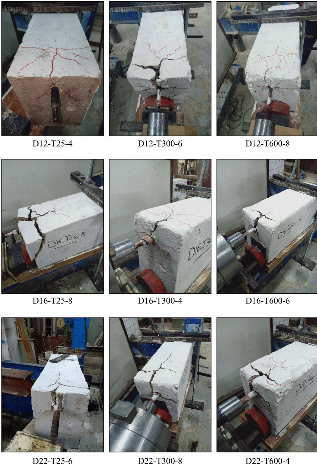
**Fig. 11** Modes of failure and cracking patterns for all tested beam-end specimens
