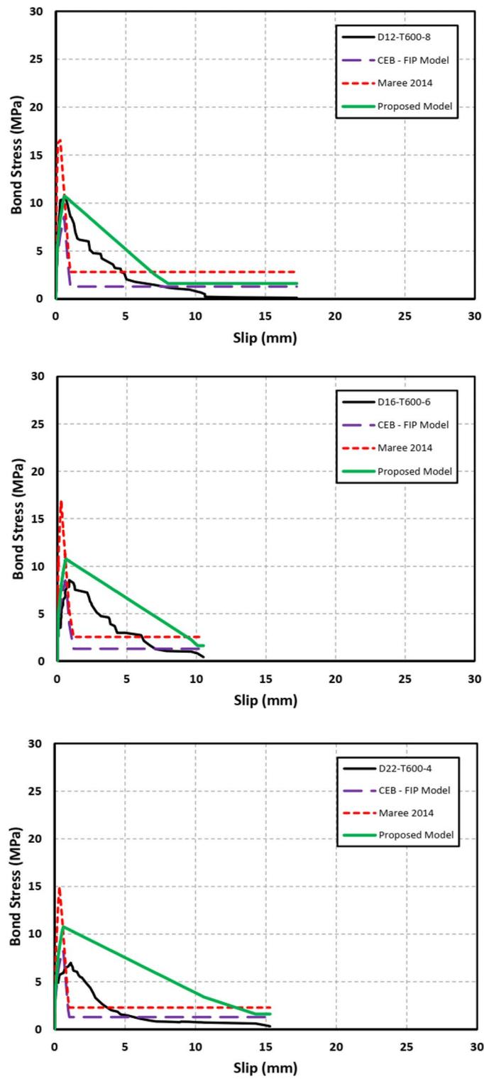
**Fig. 25** Proposed analytical versus experimental bond-slip relationships (elevated temperature of 600 °C)
