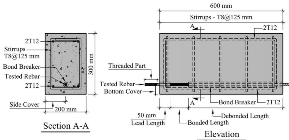
**Fig. 1** Configuration and dimensions of beam-end test specimen
