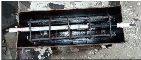
**Fig. 2** Shape of reinforcement cage and tested rebar in the mold
