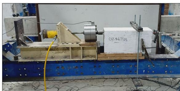
**Fig. 6** Setup of beam-end specimen test
