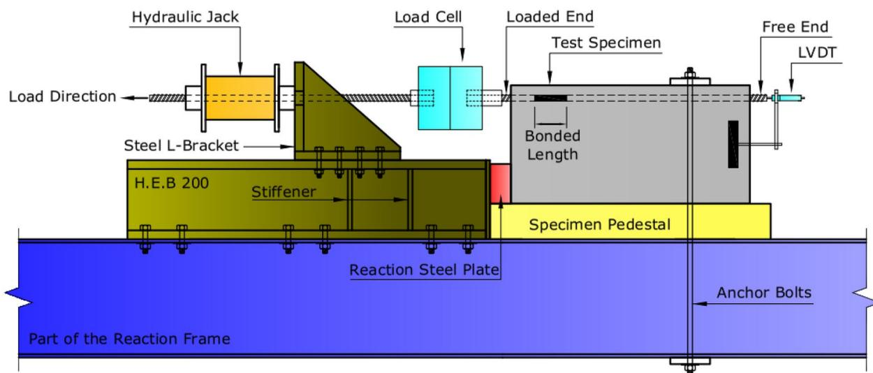
**Fig. 5** Schematic for the beam-end specimen test setup
