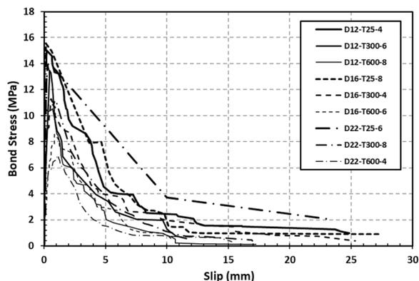
**Fig. 13** Bond stress–slip relationships of all test specimens
