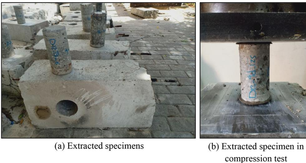
**Fig. 9** Extracting cylindrical specimens and testing them in compression
