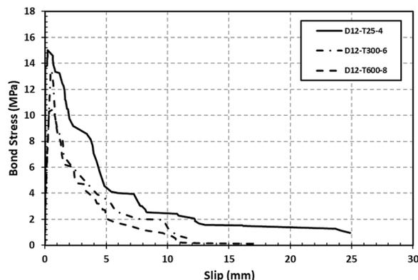
**Fig. 14** Bond stress–slip relationships of the case of 12-mm-diameter rebars
