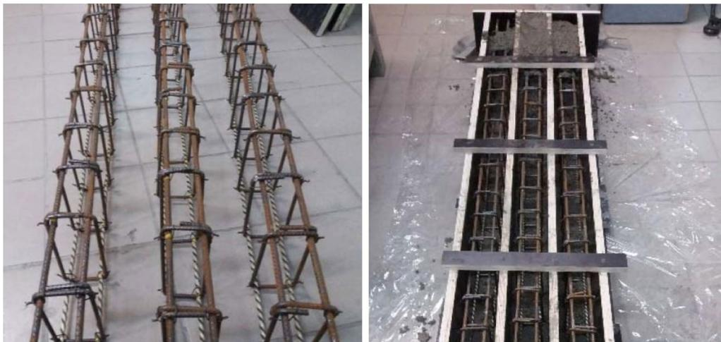
**Fig. 7** Reinforced concrete beam reinforcement
