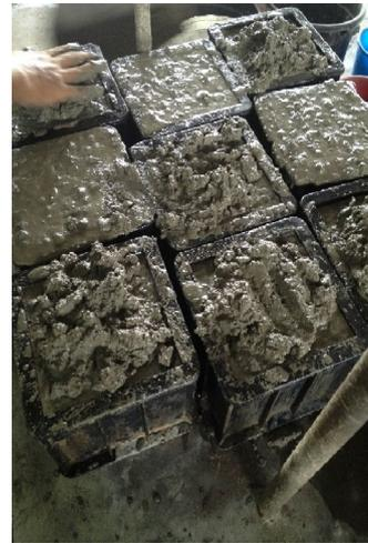
(b) Concrete compaction using a vibration table
