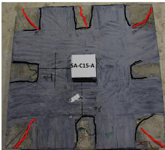
(a) Failure of specimen SA-C15-A
