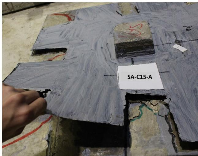
(b) Debonding of CFRP sheets in SA-C15-A
