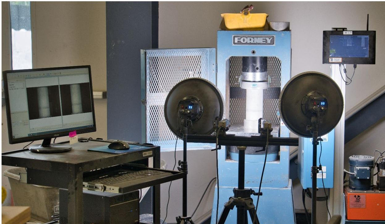
*Figure 3.3 – DIC uniaxial strain camera setup*
