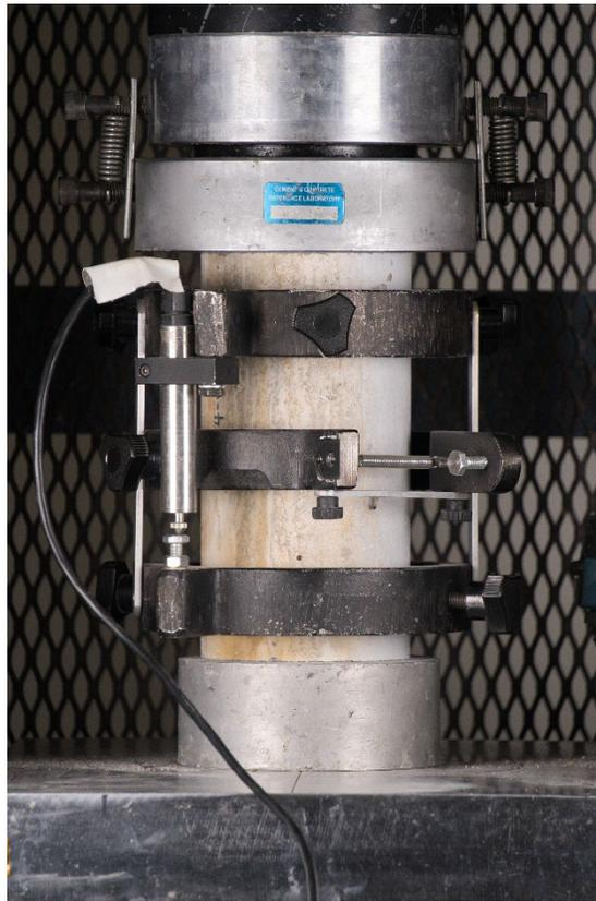
*Figure 3.4 – Compressometer MOE method setup per ASTM C469*
