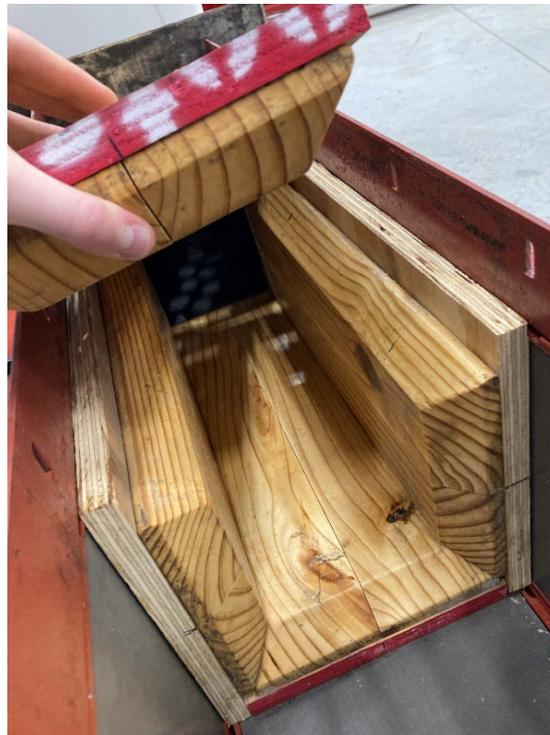
Figure 3.6 – Wooden cross-section reducing formwork
