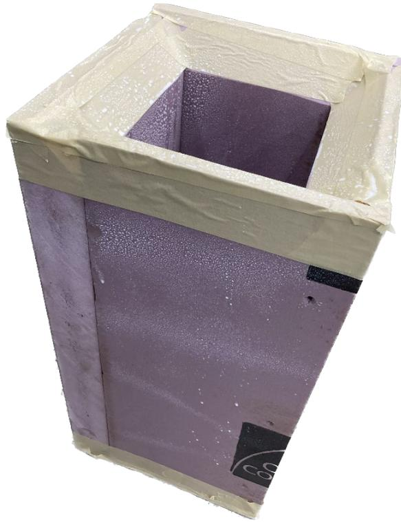
*Figure 3.7 – Foam insulation cross-section reducing formwork*
