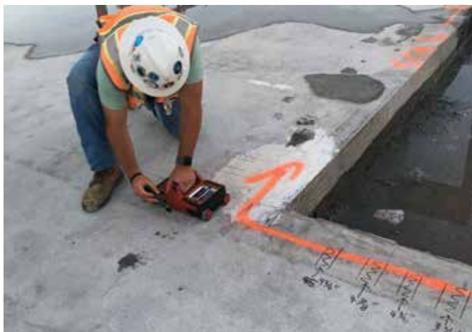
Fig. 4: Location of PT cables were marked
