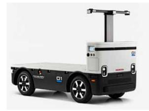
The Honda AWV employs a suite of sensors to operate autonomously, using GPS for location, radar and lidar for obstacle
