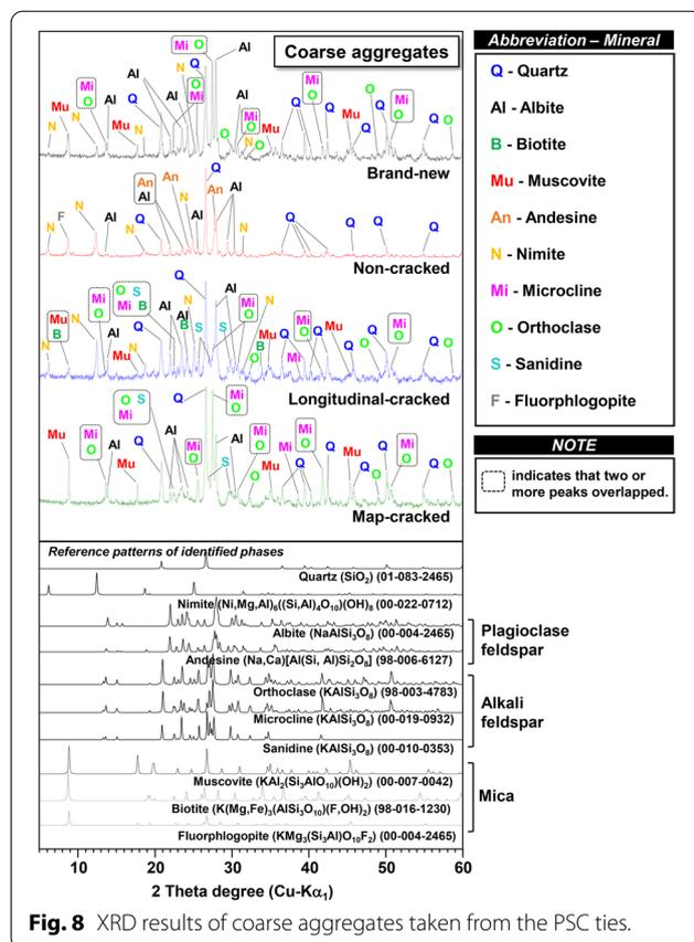
**Fig. 8** XRD results of coarse aggregates taken from the PSC ties.
