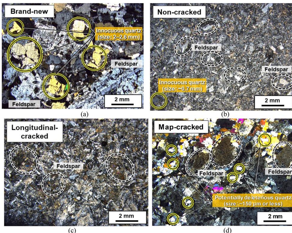
**Fig. 7** Photographs taken by polarized light microscope of coarse aggregates from **a** Brand-new, **b** Non-cracked, **c** Longitudinal-cracked, and **d** Map-cracked. Quartz grains are highlighted by a solid line of circles, and feldspar grains are indicated by dashed ellipses.
