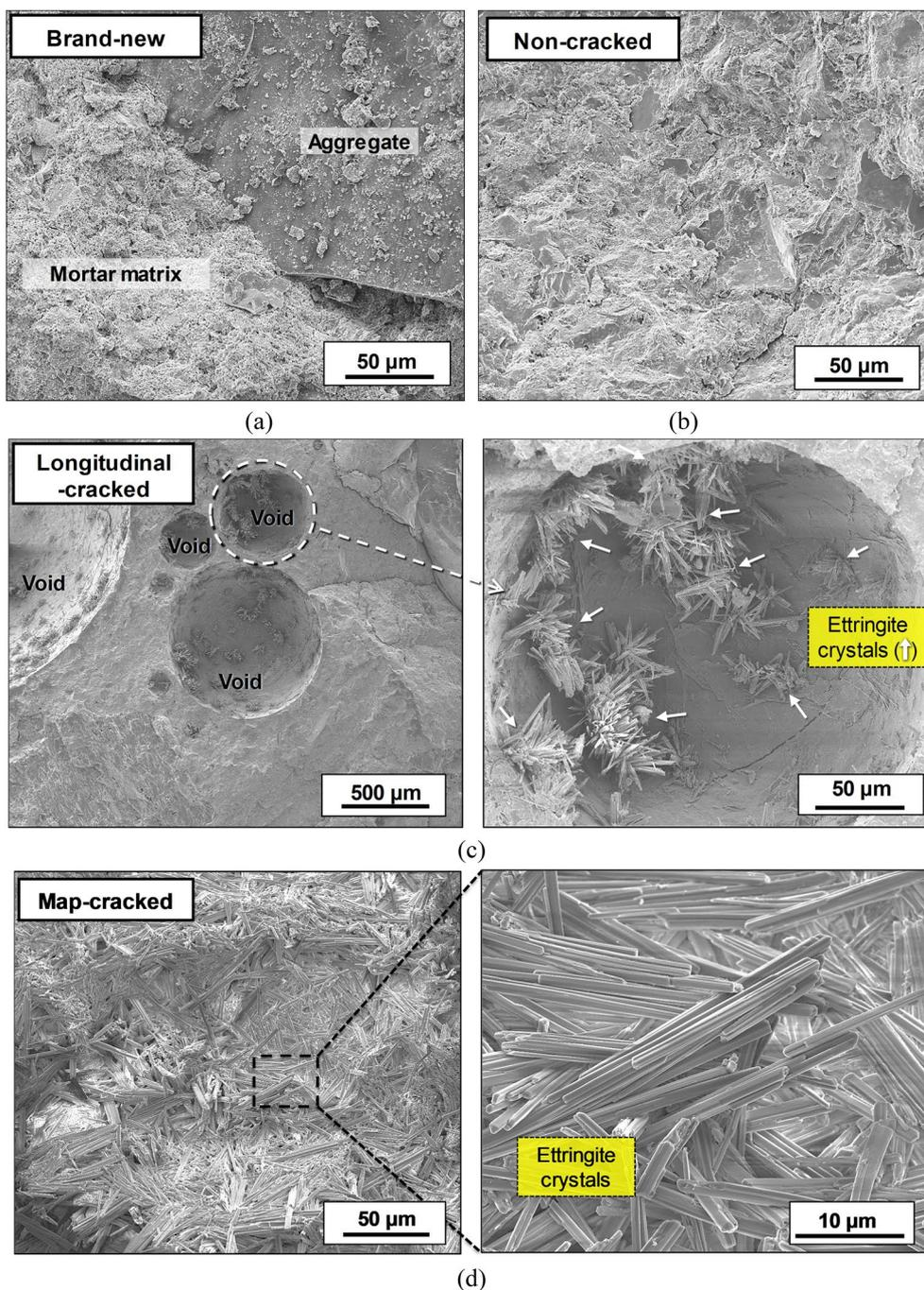
**Fig. 13** Representative microstructures of fractured surfaces for **a** Brand-new, **b** Non-cracked, **c** Longitudinal-cracked, and **d** Map-cracked in SEM SE images.
