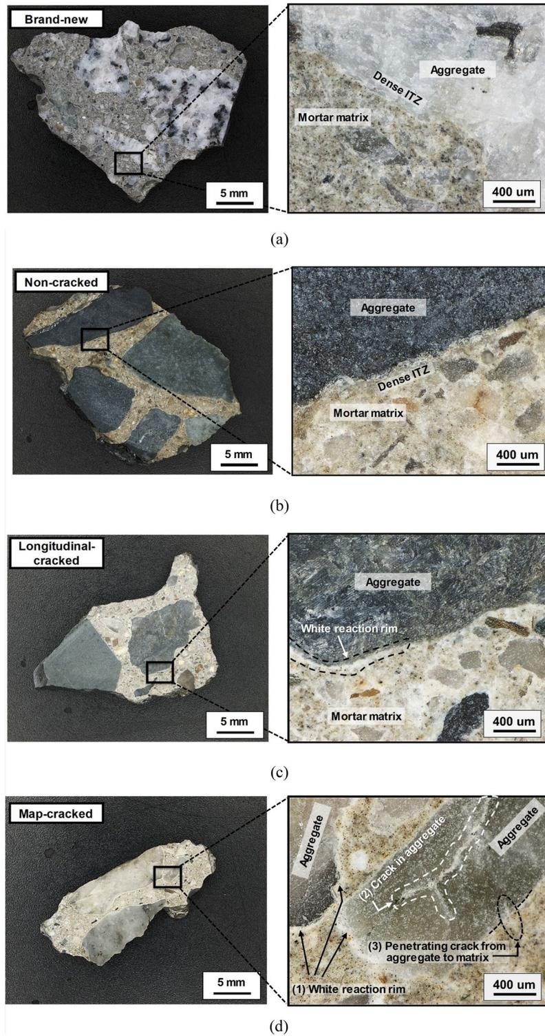
**Fig. 6** Optical microscopic images of sliced concrete samples of **a** Brand-new, **b** Non-cracked, **c** Longitudinal-cracked, and **d** Map-cracked.
