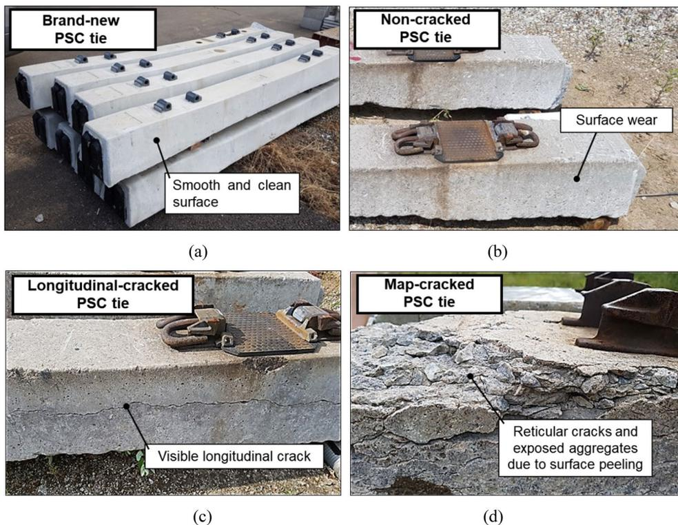
**Fig. 2** Photographs of PSC ties: **a** Brand-new, **b** Non-cracked, **c** Longitudinal-cracked, and **d** Map-cracked.
