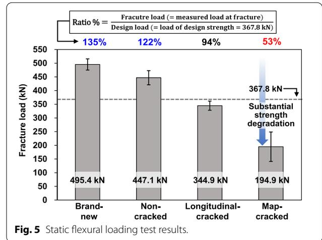
Fig. 5 Static flexural loading test results.
