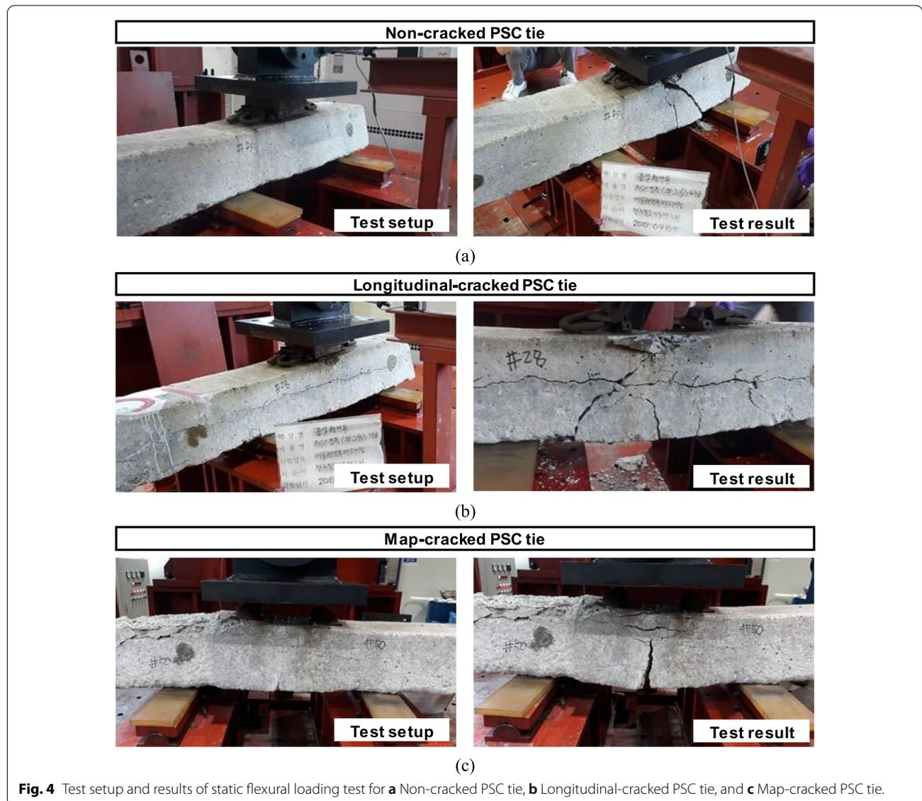
Fig. 4 Test setup and results of static flexural loading test for a Non-cracked PSC tie, b Longitudinal-cracked PSC tie, and c Map-cracked PSC tie.
