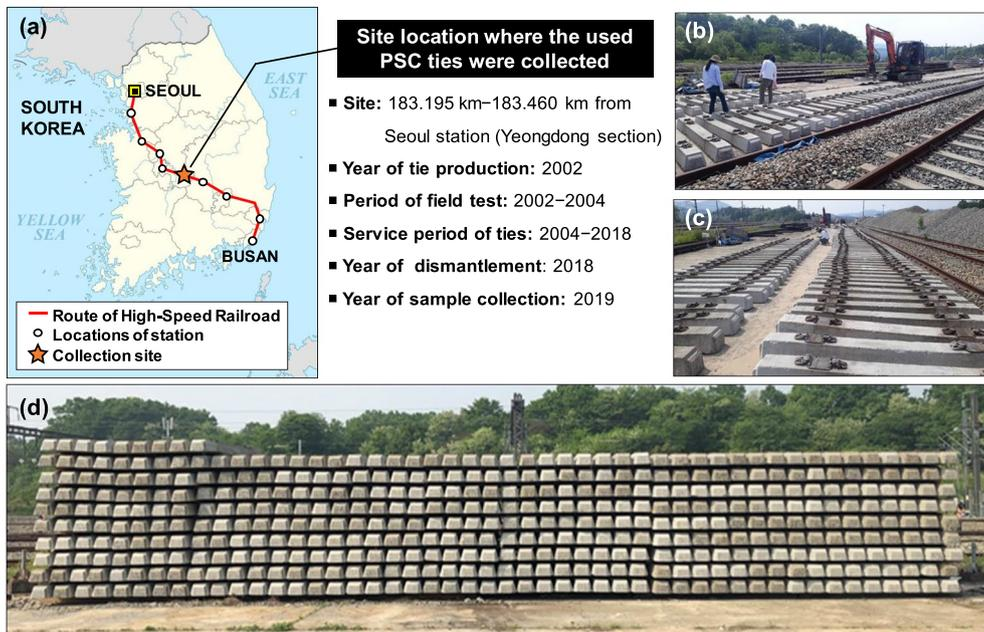
**Fig. 1** Information on the collection site and collected dismantled ties: **a** the route of Gyeongbu HSR, **b–d** photographs of collection sites and 441 collected PSC ties.
