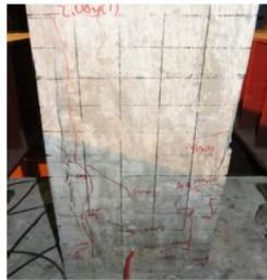
(a) Vertical splitting cracks on both sides of the back
