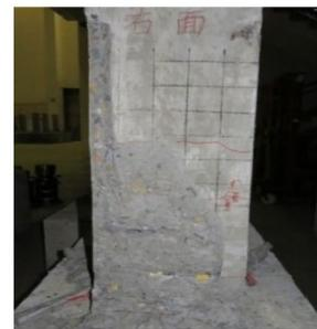
(d) The cover concrete below 50 cm on the right was crushed in one piece
