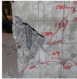
(c) Exposed longitudinal ribs at the junction of the front and left
