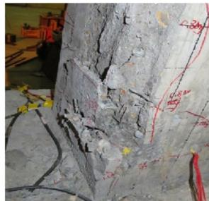
(c) The crushing area expanded to the column bottom
