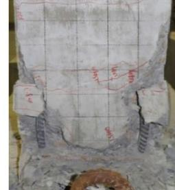
(d) The longitudinal bars on both sides of the left side were exposed and buckled
