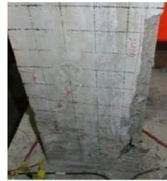
(b) Crushed edges at the junction between the back and the right
