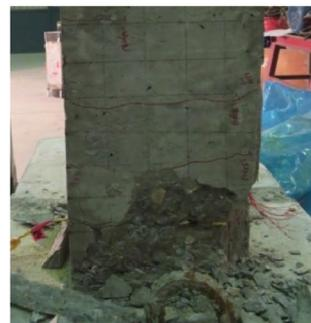
(d) Severely crushed in the plastic hinge zone of concrete on the right after failure
