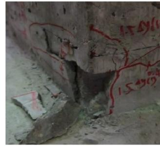
(b) The cover concrete of the column bottom spalled
