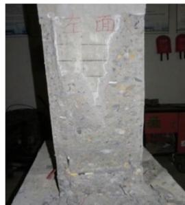
(c) The cover concrete below 70 cm on the left was crushed in one piece
