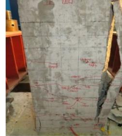
(b) Split cracks and uplift of the cover concrete on the right
