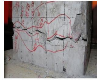
(b) The main crack on the left and the uplift of the cover concrete
