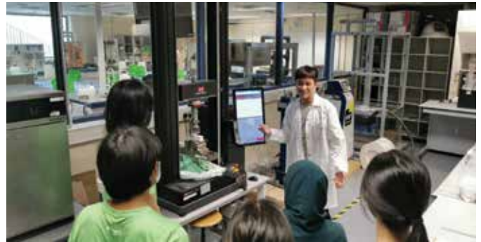
Flexural testing of clay beams using an Instron universal testing machine
