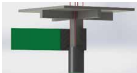
Fig. 3: Installation of laminates around the column to create a shell
