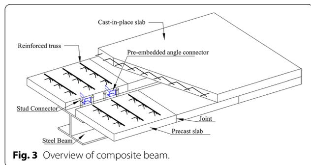
**Fig. 3** Overview of composite beam.
