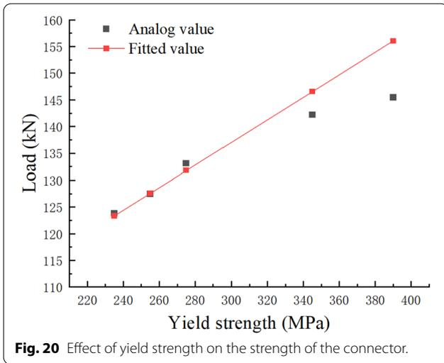
Fig. 20 Effect of yield strength on the strength of the connector.
