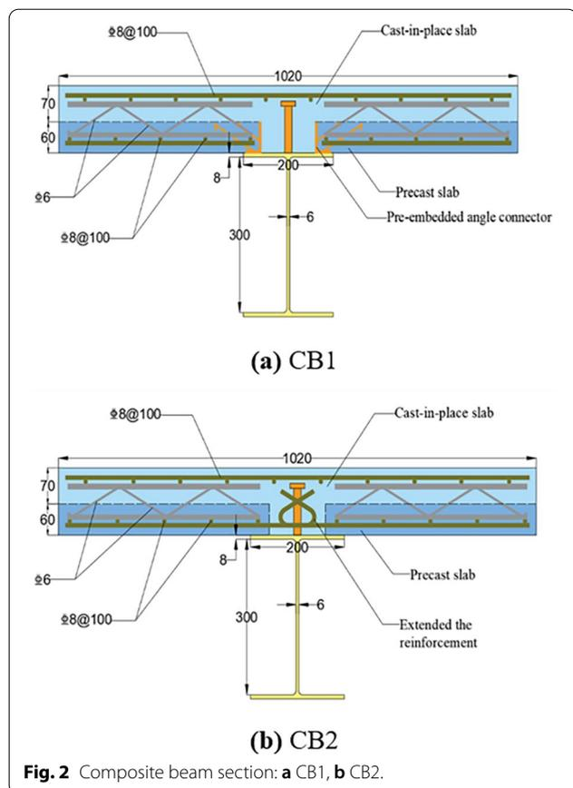
**Fig. 2** Composite beam section: **a** CB1, **b** CB2.
