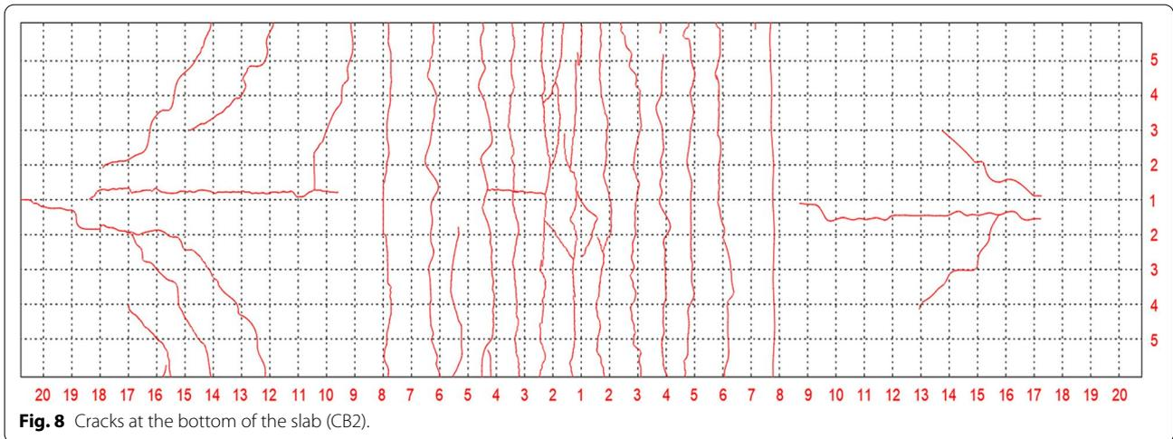
the load was increased to 60 kN–76 kN, the first crack appeared at the mid-span of the two specimens. This crack eventually became the fastest developing and the widest "main crack". With the load increased, new cracks kept developing along the length of the slab. At the same time, cracks at the mid-span kept developing and gradually increased in width. Eventually, it developed into a crack through the concrete slab.
