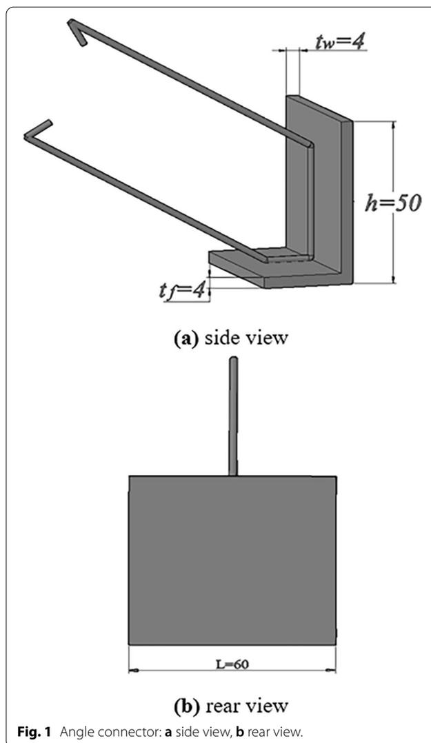
**Fig. 1** Angle connector: **a** side view, **b** rear view.
