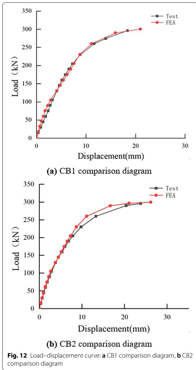
large plastic deformation or even shearing at both the root of the connector and the weld during the test (Qiu et al., 2021). As a result, shear damage and flexible damage in ABAQUS were used to simulate the degradation of the strength and stiffness of the angle connector (Liu, 2020). The rest of the steel material property models were consistent with the above.
