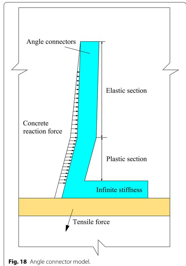
Fig. 18 Angle connector model.
