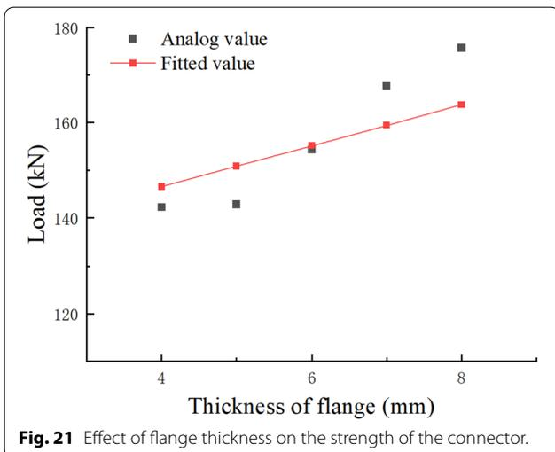
Fig. 21 Effect of flange thickness on the strength of the connector.
