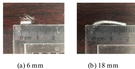
**Fig. 1** PVA fibers of different lengths.
