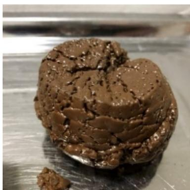
**Fig. 4** Attapulgite calcined at 800 °C for 2 h (fully sintered).
