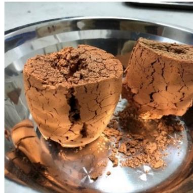
**Fig. 3** Attapulgite calcined at 700 °C for 2 h (fully sintered).
