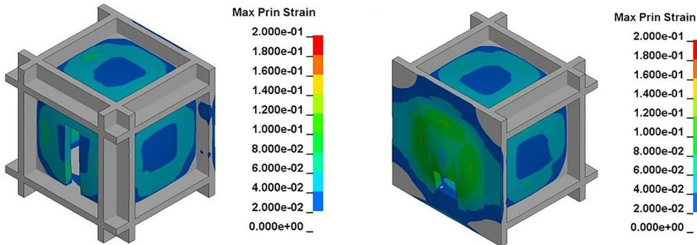
(b) Numerical simulation results without afterburn
