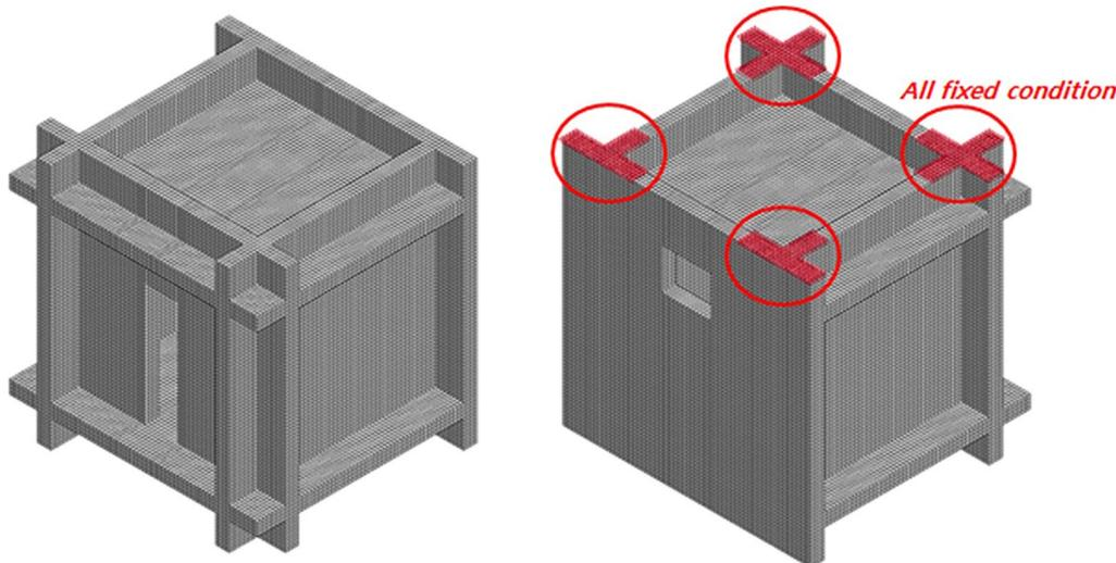
**Fig. 18** Boundary condition of the reinforced concrete room.
