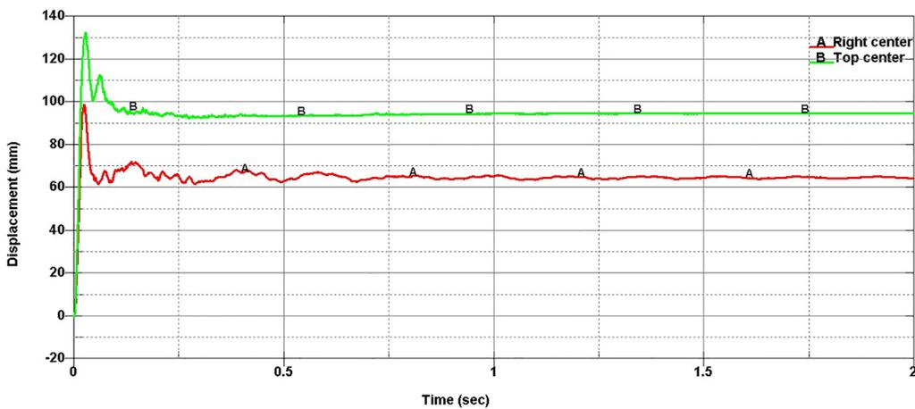
**Fig. 8** Displacement measurement data (TNT 2 kg).
