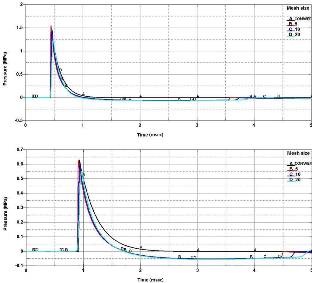
**Fig. 11** Pressure behavior with time at distances of 1 m (top) and 1.5 m (bottom) from the 2 kg TNT detonation position.
