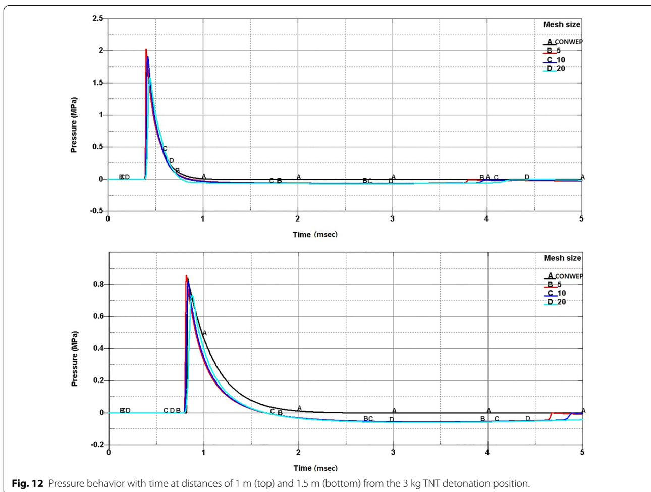
Fig. 12 Pressure behavior with time at distances of 1 m (top) and 1.5 m (bottom) from the 3 kg TNT detonation position.
