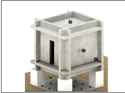
**Fig. 3** Reflection pressure sensor locations.
