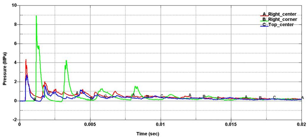
**Fig. 7** Pressure measurement data (TNT 2 kg).
