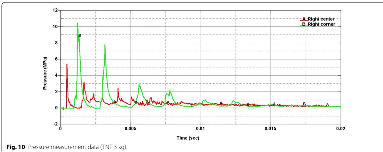
**Fig. 10** Pressure measurement data (TNT 3 kg).
