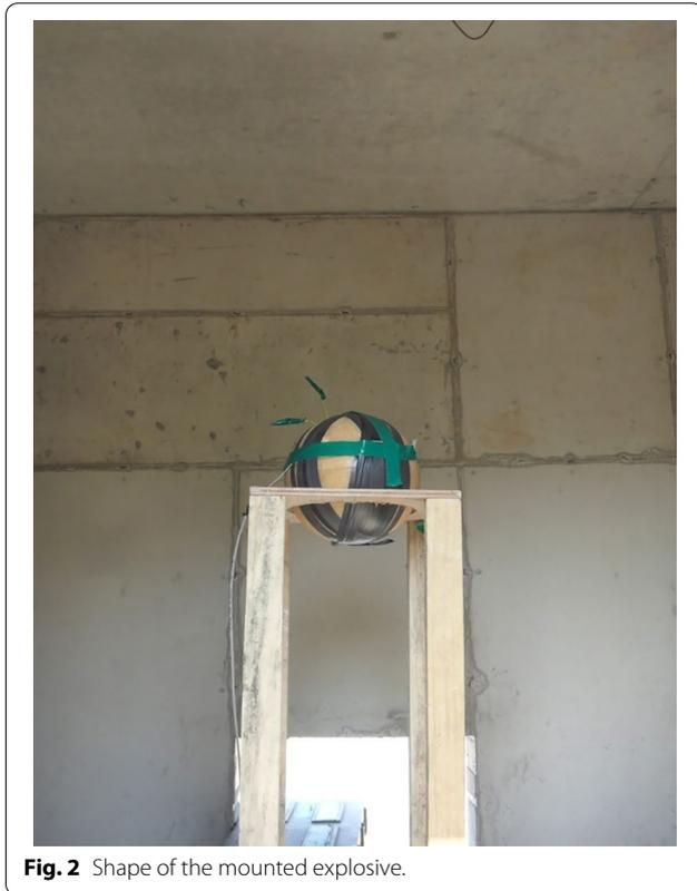
**Fig. 2** Shape of the mounted explosive.
