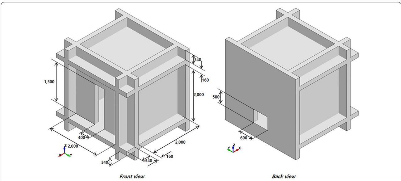
**Fig. 15** Reinforced concrete room shape.
