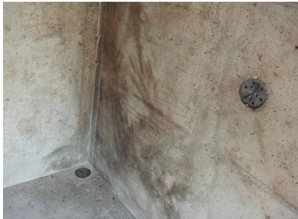
**Fig. 4** Reflective pressure sensor installation shape.
