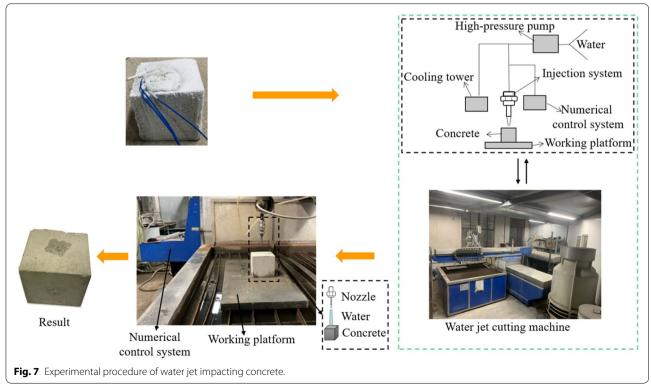
of C30 concrete samples after  $LN_2$  cold shock of 5 min and 10 min are selected as the research objects. The experimental procedure is demonstrated in Fig. 7.
