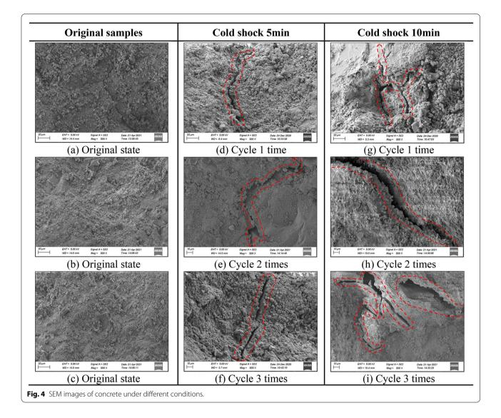
It can be concluded that micro-cracks were generated in two forms: one is that a large number of new cracks were derived, the other is that the original cracks propagated and interpenetrated to generate overall destruction of the concrete structure to a large extent.
