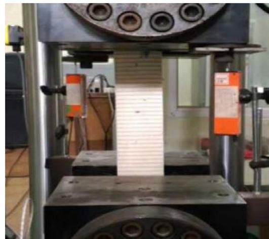
(b) Tension test of HF strand in progress
