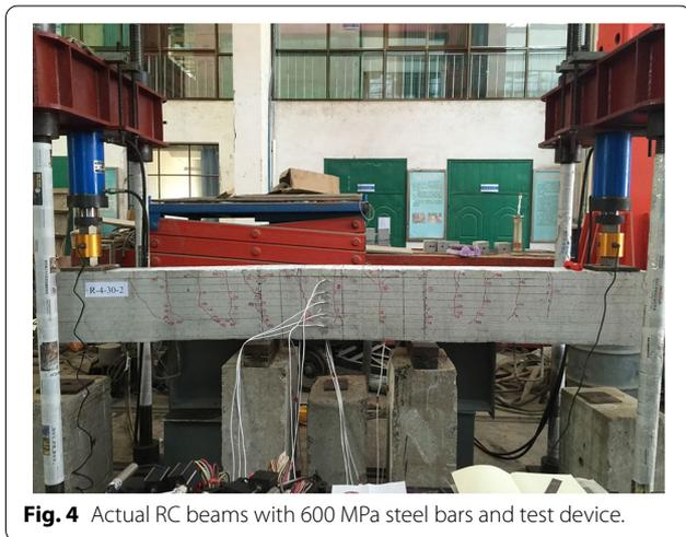
**Fig. 4** Actual RC beams with 600 MPa steel bars and test device.
