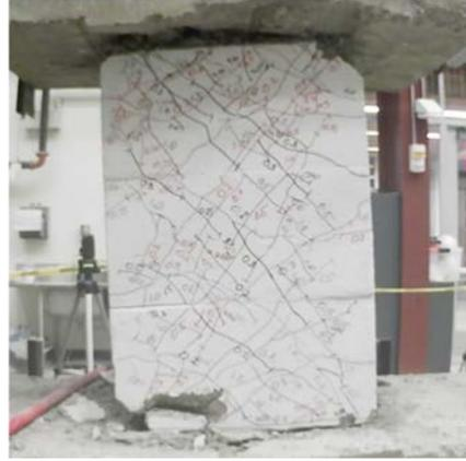
Figure C.18 – D100-1.5 at -6% chord rotation, second cycle
