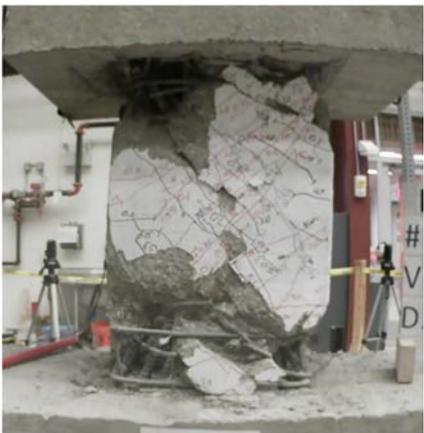
Figure C.9 – D80-1.5 at +8% chord rotation, first cycle
