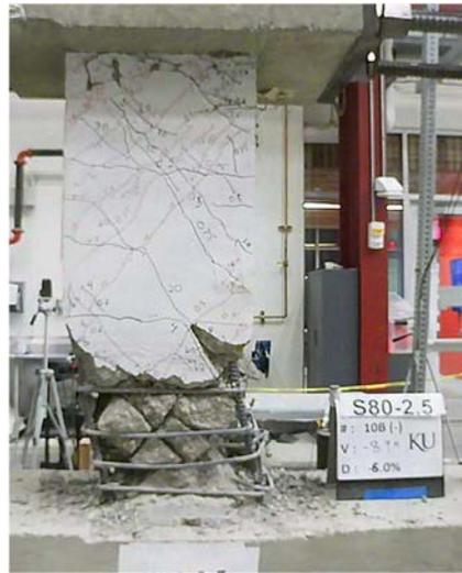
Figure C.101 – P80-2.5 at -6% chord rotation, second cycle
