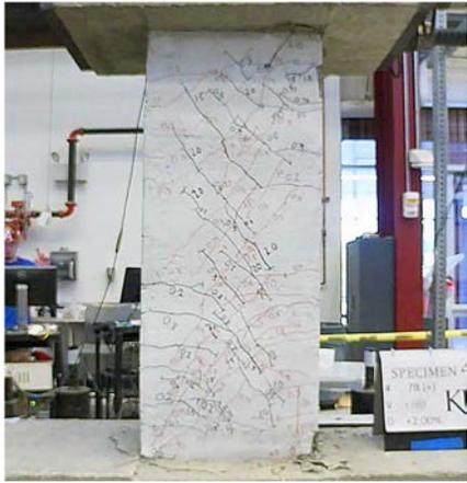
Figure C.30 – D80-2.5 at +2% chord rotation, second cycle
