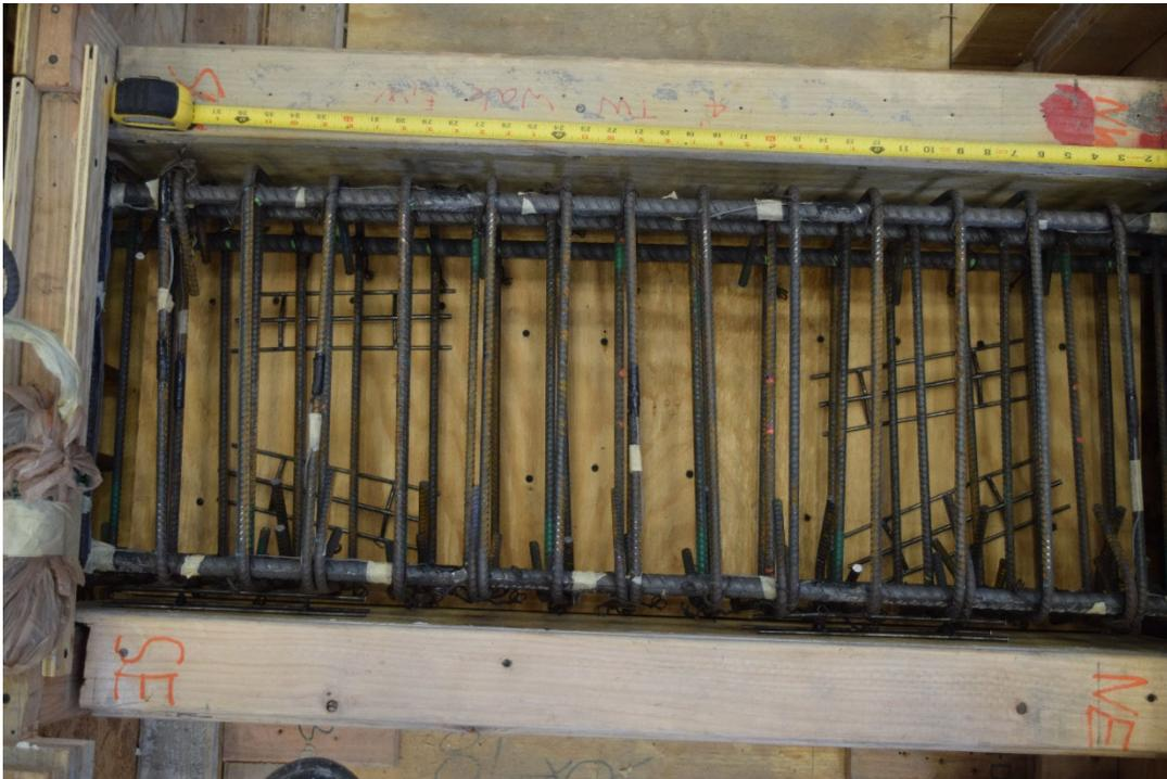
Figure B.4 – Coupling beam reinforcement, P100-2.5
