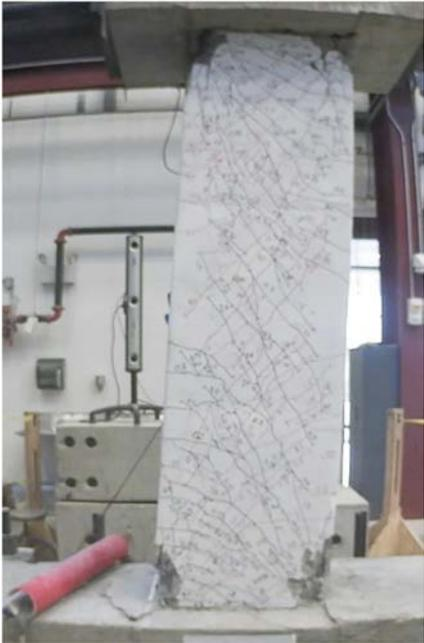
Figure C.66 – D80-3.5 at +6% chord rotation, second cycle
