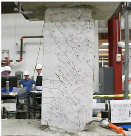
Figure C.32 – D80-2.5 at +4% chord rotation, second cycle
