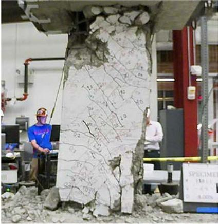
Figure C.38 – D80-2.5 at +10% chord rotation, first cycle
