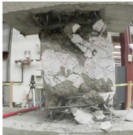
Figure C.10 – D80-1.5 at -8% chord rotation, first cycle
