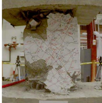
Figure C.8 – D80-1.5 at -6% chord rotation, second cycle
