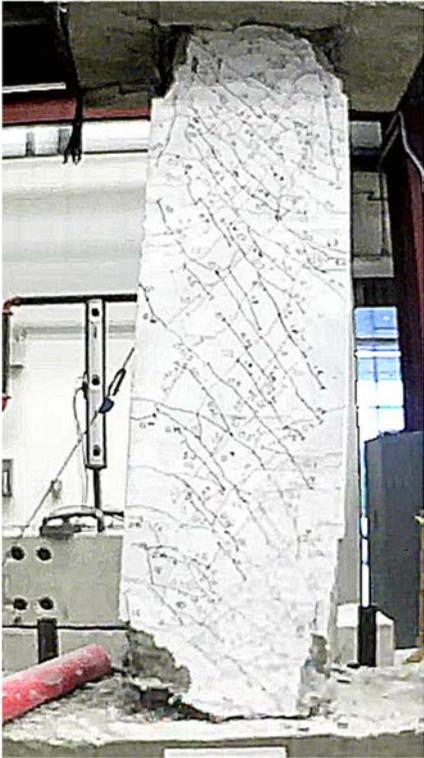
Figure C.78 – D100-3.5 at +6% chord rotation, second cycle
