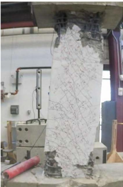
Figure C.68 – D80-3.5 at +8% chord rotation, second cycle
