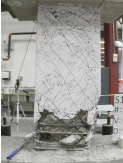
Figure C.108 – P100-2.5 at +6% chord rotation, second cycle
