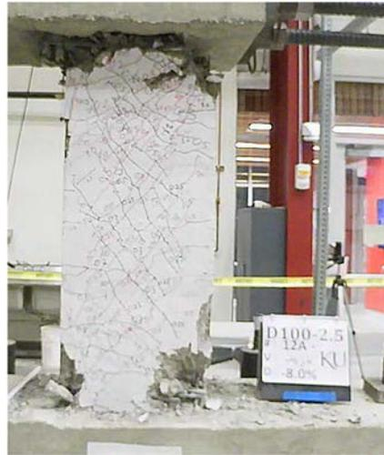
Figure C.49 – D100-2.5 at -8% chord rotation, first cycle
