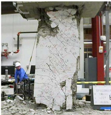
Figure C.36 – D80-2.5 at +8% chord rotation, second cycle
