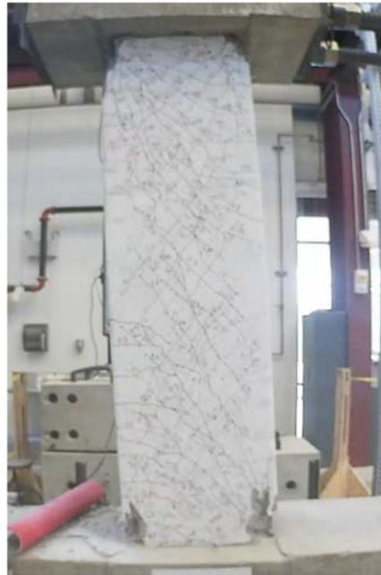
Figure C.65 – D80-3.5 at -4% chord rotation, second cycle
