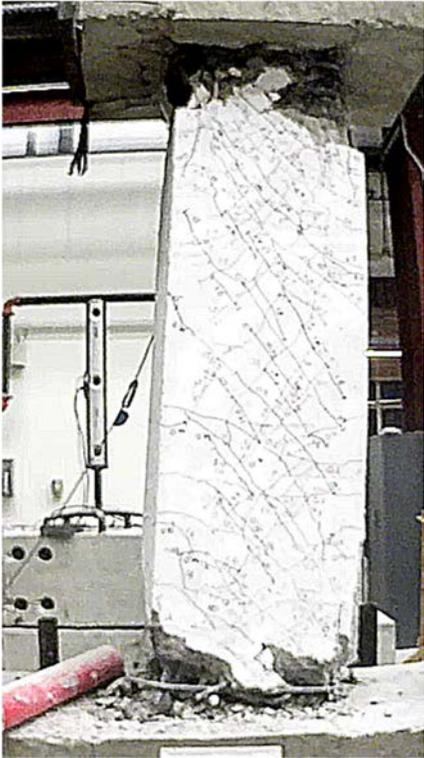
Figure C.82 – D100-3.5 at +10% chord rotation, first cycle
