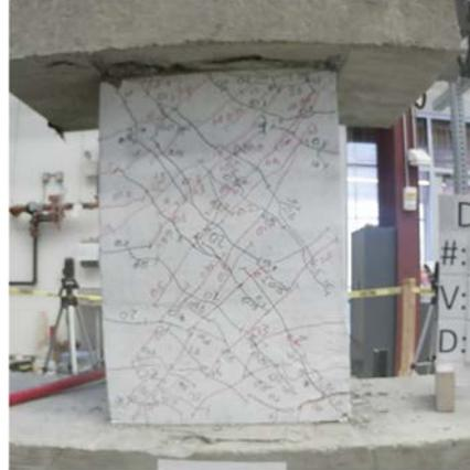
Figure C.4 – D80-1.5 at -2% chord rotation, second cycle
