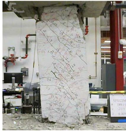
Figure C.35 – D80-2.5 at -6% chord rotation, second cycle
