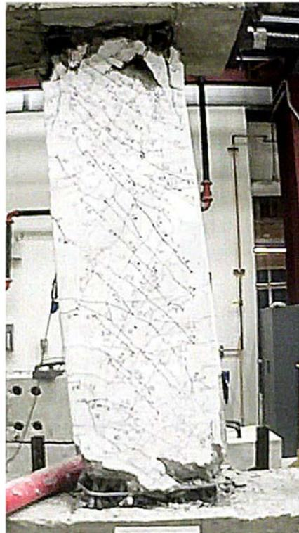
Figure C.81 – D100-3.5 at -8% chord rotation, second cycle
