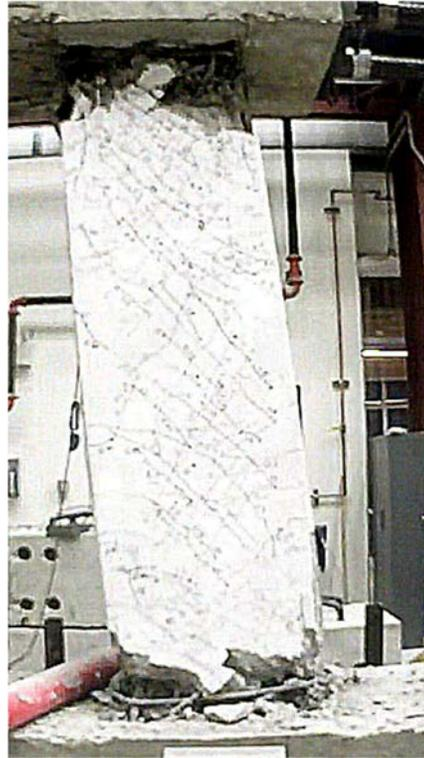
Figure C.83 – D100-3.5 at -10% chord rotation, first cycle
