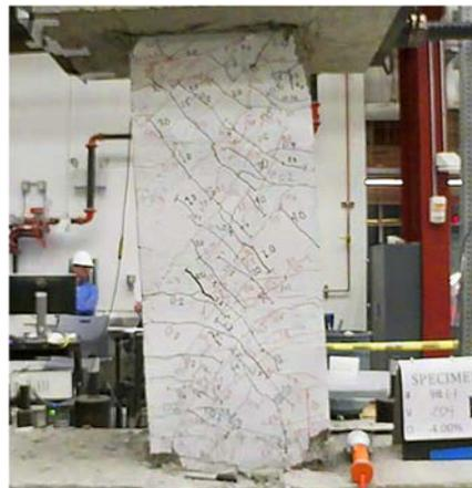
Figure C.33 – D80-2.5 at -4% chord rotation, second cycle
