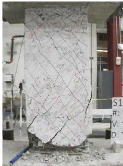
Figure C.107 – P100-2.5 at -4% chord rotation, second cycle
