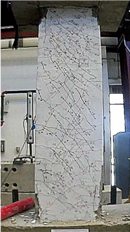
Figure C.74 – D100-3.5 at +2% chord rotation, second cycle
