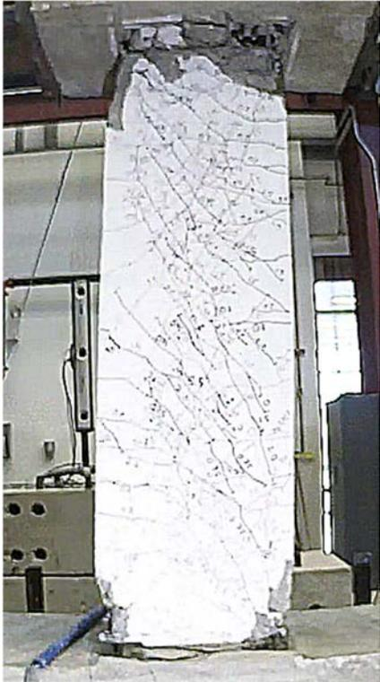
Figure C.90 – D120-3.5 at +6% chord rotation, second cycle
