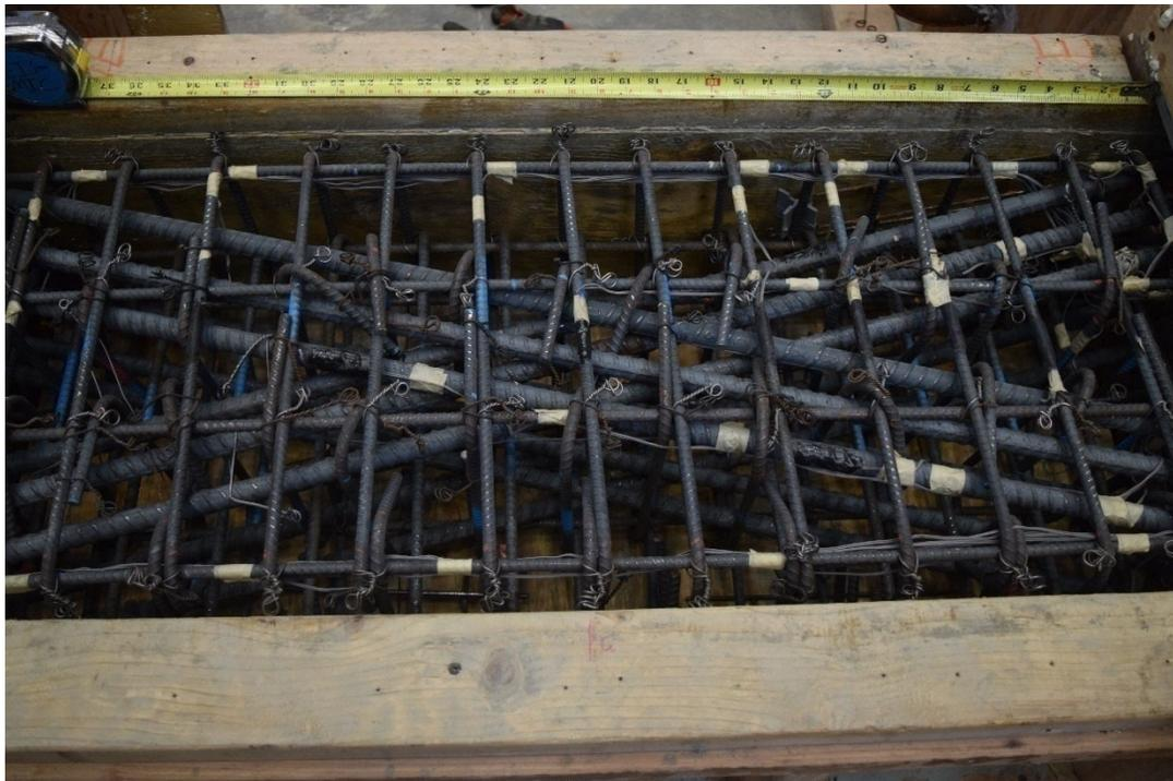
Figure B.2 – Coupling beam reinforcement, D120-2.5
