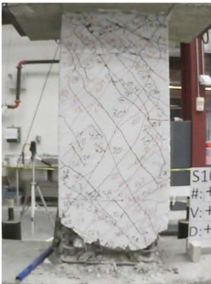
Figure C.106 – P100-2.5 at +4% chord rotation, second cycle
