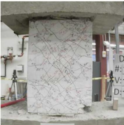
Figure C.5 – D80-1.5 at +4% chord rotation, second cycle
