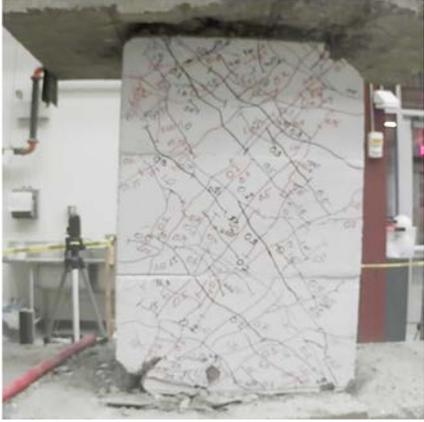
Figure C.17 – D100-1.5 at +6% chord rotation, second cycle
