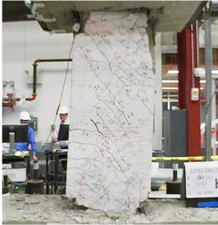
Figure C.34 – D80-2.5 at +6% chord rotation, second cycle
