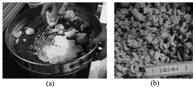
Fig. 4—Granulation of SM for ensuring of continuous material feeding: (a) sieves used for manual granulation of SM; and (b) granulated SM (scale in cm).
