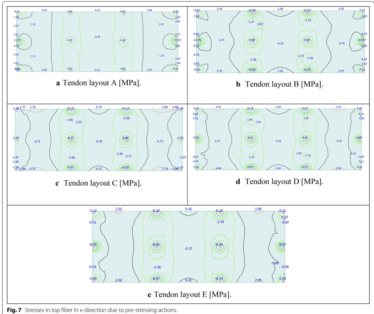
**Fig. 7** Stresses in top fiber in x-direction due to pre-stressing actions.
