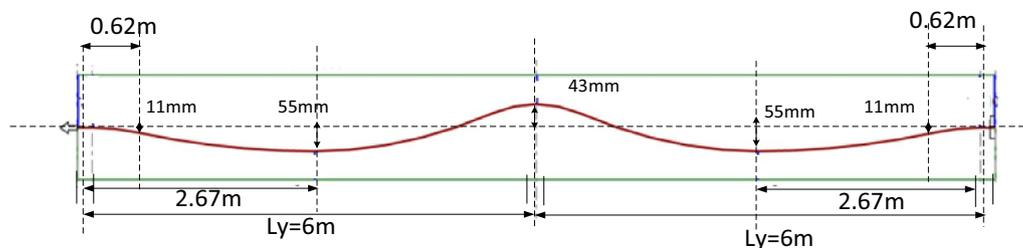
**Fig. 3** Tendon profile and the eccentricities when  $L_y=6$  m.
