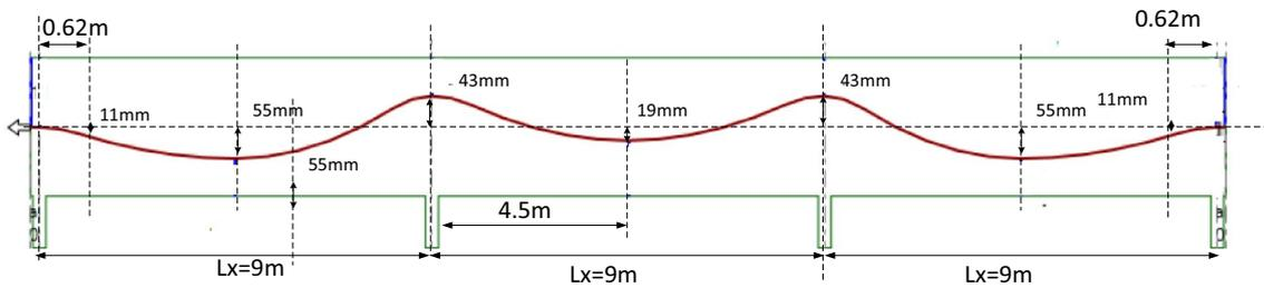
**Fig. 4** Tendon profile and the eccentricities when  $L_x = 9$  m.
