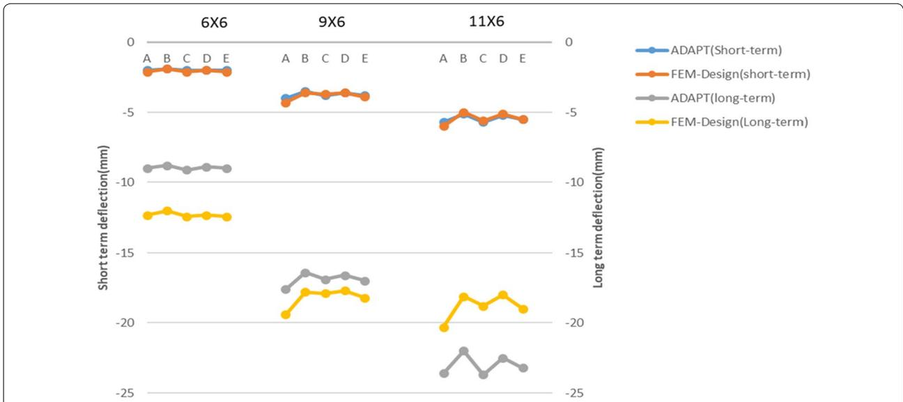
**Fig. 6** Tendon layout analysis—deflections in millimeters.
