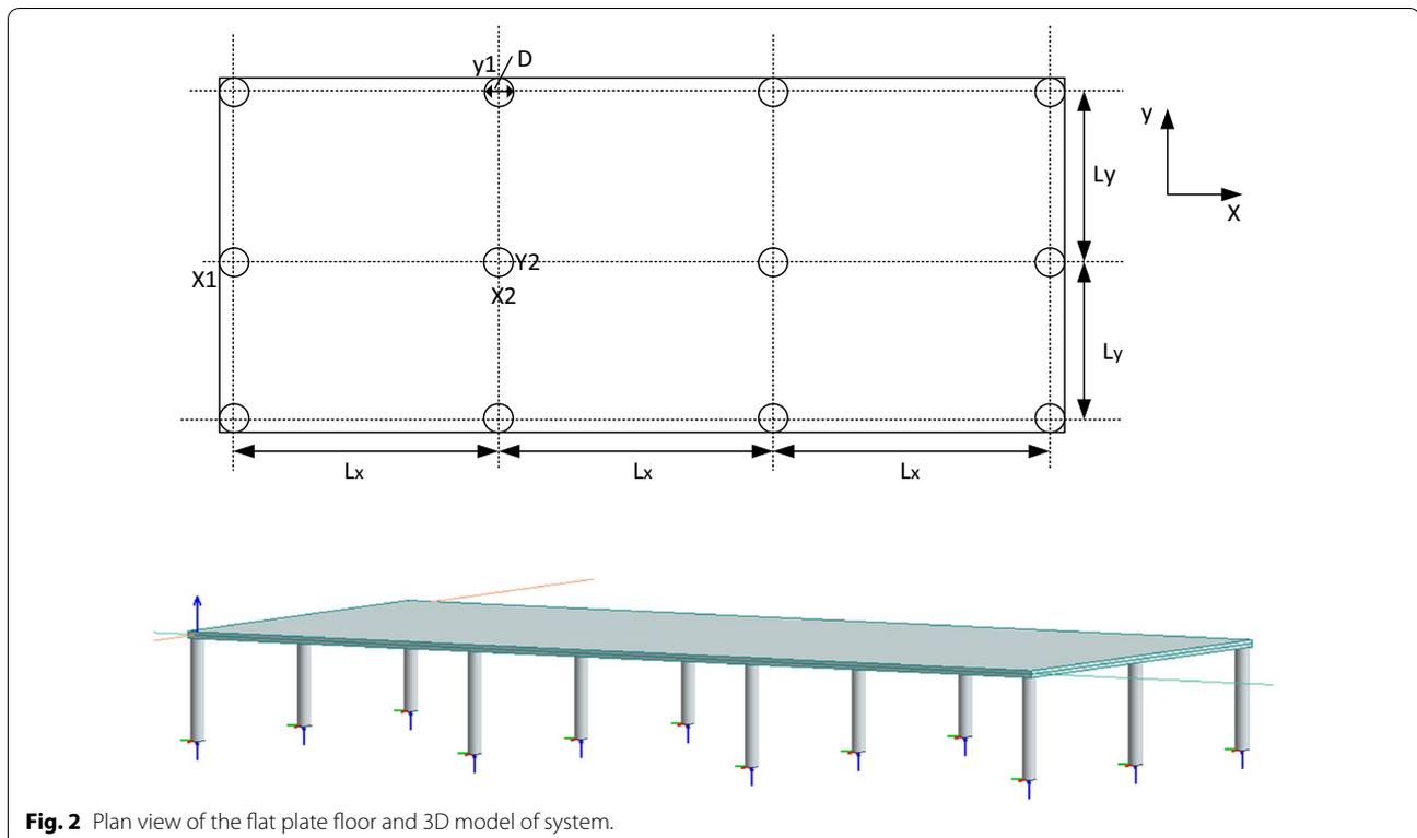
**Fig. 2** Plan view of the flat plate floor and 3D model of system.
