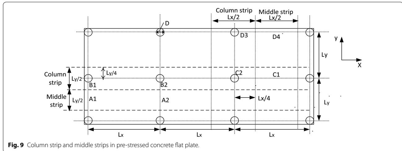
**Fig. 9** Column strip and middle strips in pre-stressed concrete flat plate.
