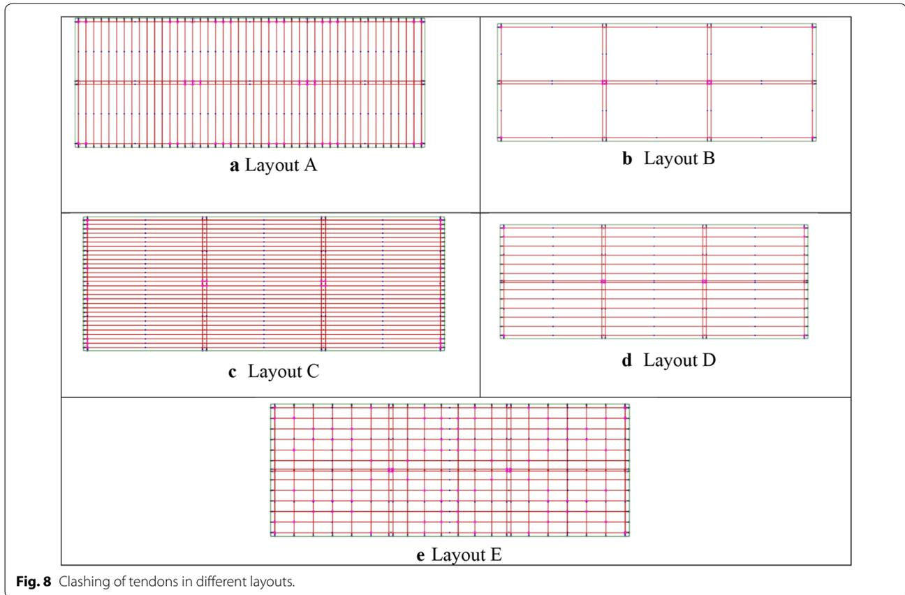
**Fig. 8** Clashing of tendons in different layouts.
