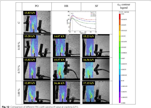
figures that the load-resisting capacities of different fibre types lie in different ranges after cracking. The resistance range at 0.5 mm CMOD for SynFRC is from 4 kN to 7 kN (Fig. 9), whereas, it ranges from 6 kN to 10 kN for HFRC (Fig. 10) and from 10 kN to 15 kN for SFRC (Fig. 11). This showcases how hybridisation of two different types of fibres helps at service limit state. These graphs confirm that peak loads tend to increase with  $V_{\theta}$  except for SynFRC.
