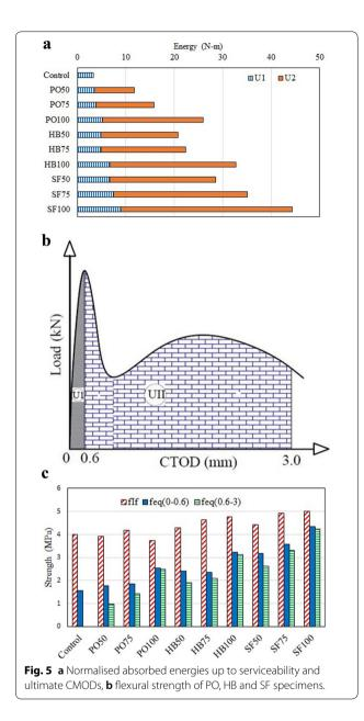
but the ratio of equivalent strengths. The results show that synthetic and hybrid fibres are more effective at higher crack widths corresponding to the ultimate state.
