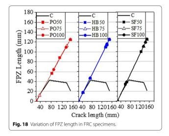
SF fibres increased linearly up to 130 mm, as shown in Fig. 18. A linear variation of FPZ length with crack length was observed for all the fibre volume fractions and fibre types. No appreciable change in variation of FPZ length was observed due to the change in fibre dosage and fibre
