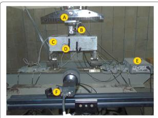
**Fig. 2** Fracture test setup: **a** loading beam; **b** displacement sensor; **c** notched specimen; **d** AE sensors; **e** wave actuator; **f** camera.
