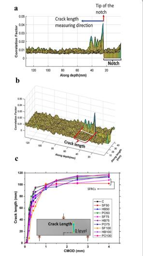
**Fig. 14** Illustration of measurement of crack length from the notch tip and graphs of crack length Vs. CMOD: **a** variation of correlation factor along the depth of the specimen HB100 at 0.2 mm CMOD; **b** measurement of crack propagation from the notch; **c** crack length vs. CMOD graphs of all specimens.
