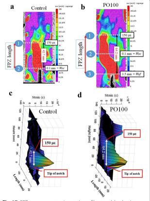
**Fig. 17** FPZ measurement using strain profile at peak load point: **a** idealisation of FPZ, **b** control beam, **c** PO100 beam.
