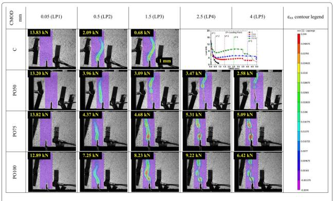
Fig. 9 Comparison of strains of SynFRC with different fibre dosages at considered CMODs.
