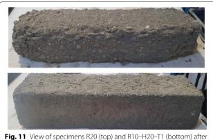
Fig. 11 View of specimens R20 (top) and R10–H20–11 (botto 108 cycles.
