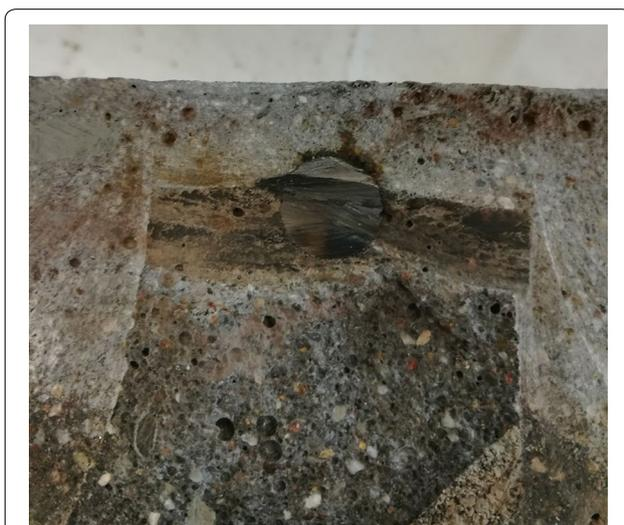
**Fig. 7** Photo taken after cutting specimen number 10, at the end of its corrosion test. Steel corrosion products have concentrated on top of the steel rebar and are filling the open crack produced by corrosion.
