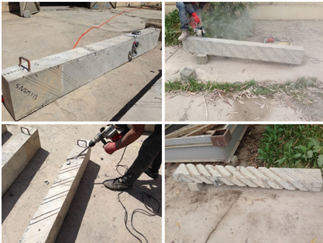
Fig. 3 Continuous spiral NSN groove preparation.
