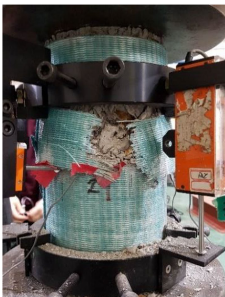
a C-P2-150mm: FRP rupture
