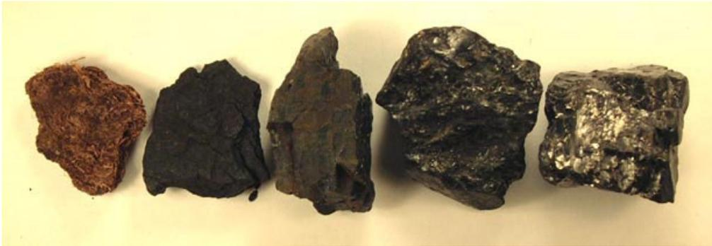
**Figure 2-3.** From left to right: peat, lignite, sub-bituminous, bituminous, and anthracite coal [14]
