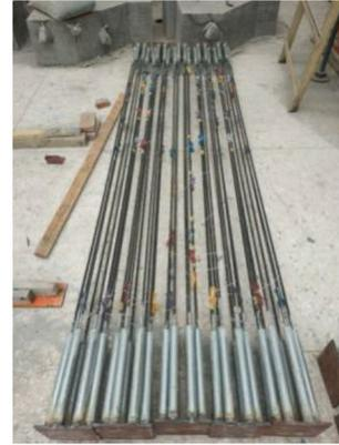
**Fig. 2** Anchorage setup for CFRP bar.
