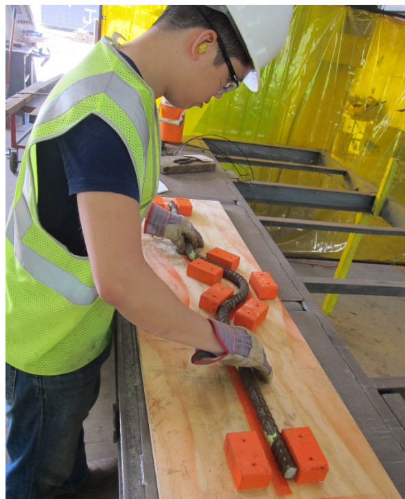
Figure 4: Verifying bend specimen tolerance
