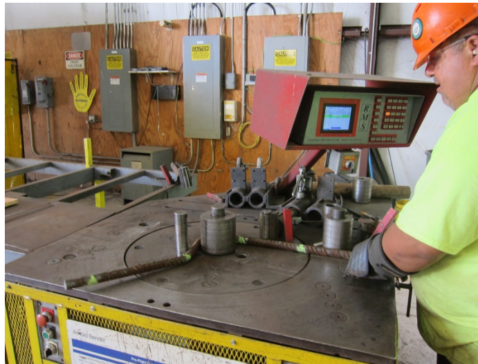
Figure 3: RMS Arnold Bender used to bend specimens
