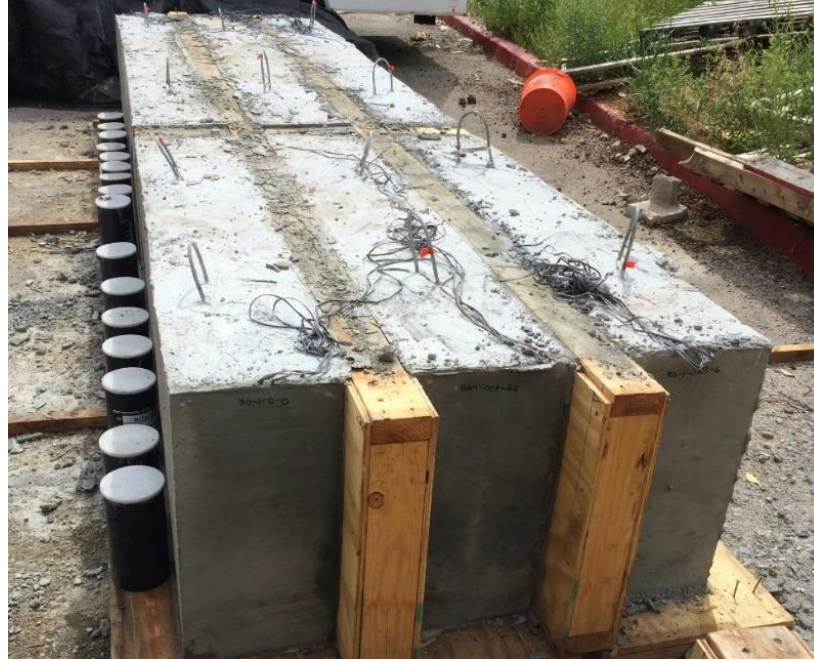
Figure 3-13: Concrete Beams and Cylinders after 28 days of Curing
