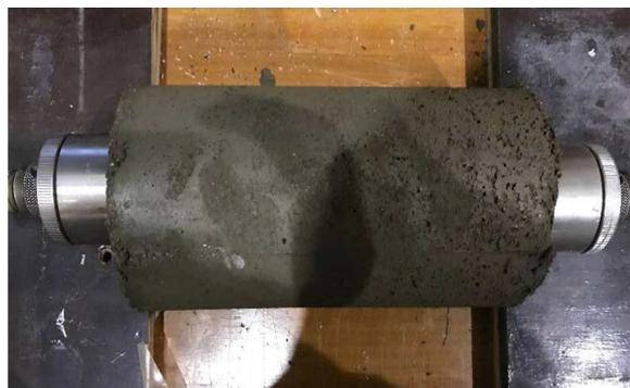
(a) Ultrasonic Pulse Velocity Method
