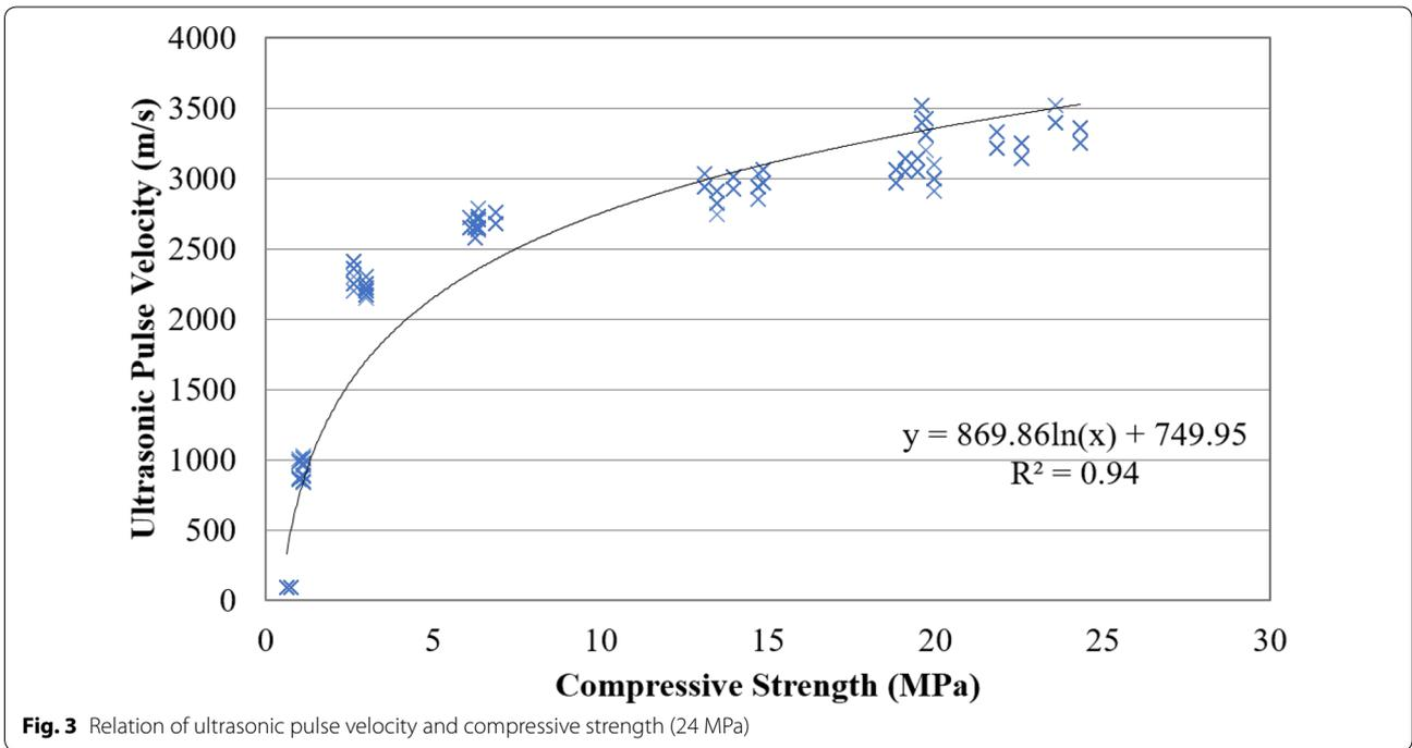
75.00% 672 h, respectively. Figure 6 shows that as for the correlation between compressive strength and wave velocity, as wave speed increased, compressive
