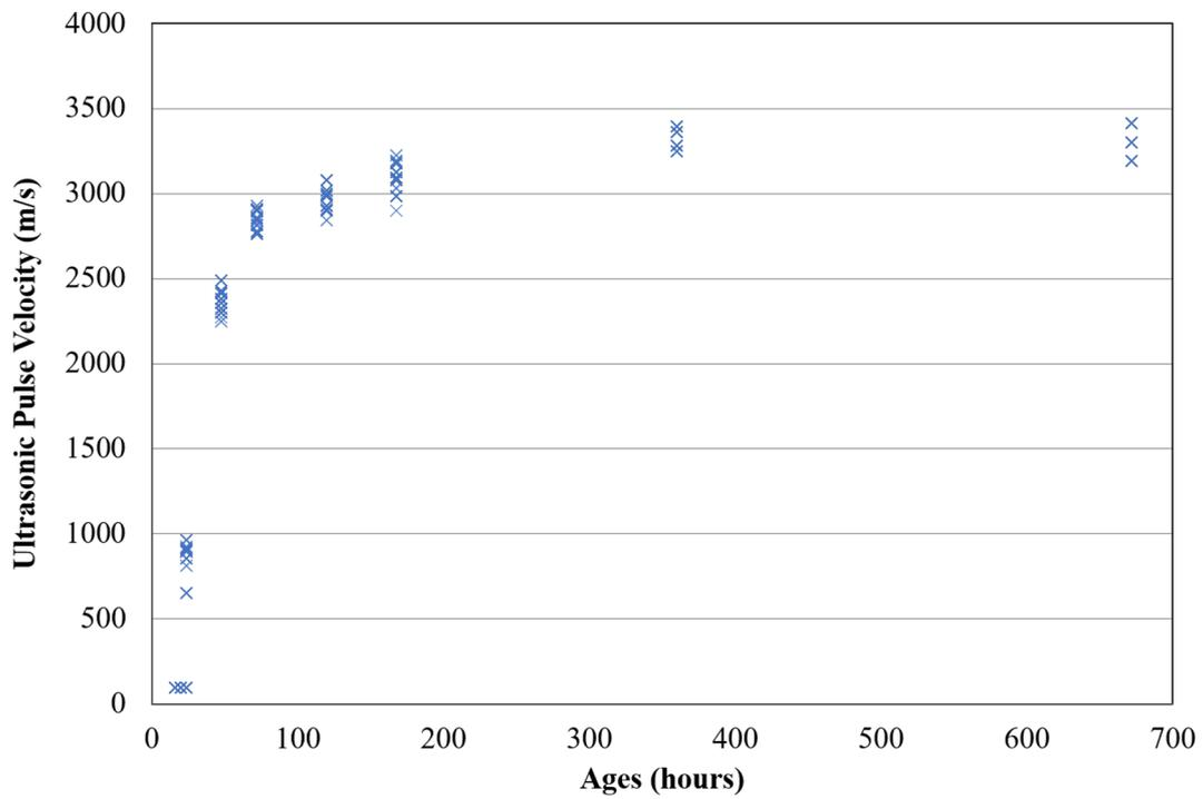
**Fig. 4** Ultrasonic pulse velocity with ages (30 MPa)
