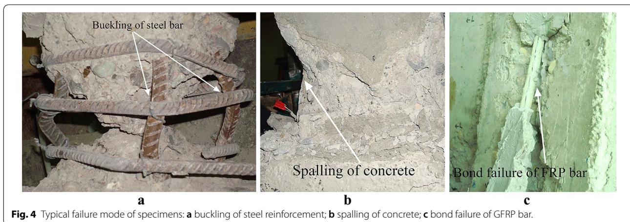
**Fig. 4** Typical failure mode of specimens: **a** buckling of steel reinforcement; **b** spalling of concrete; **c** bond failure of GFRP bar.
