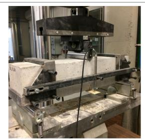
**Fig. 5** Three-point bending test of a notched specimen according to the RILEM work-of-fracture method.
