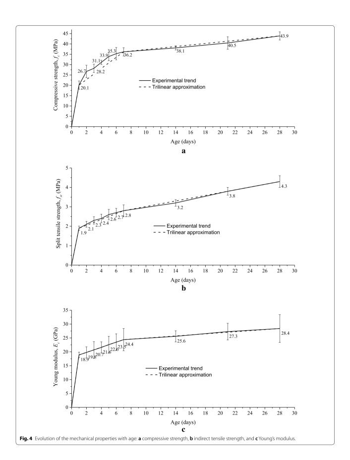
allows to reduce the number of tests needed to determine the evolution of  $f_c$ ,  $f_{st}$ , and  $E_c$  with age. In the case of the Young's modulus (Fig. 4c), the real trend and the trilinear approximation are practically coincident.
