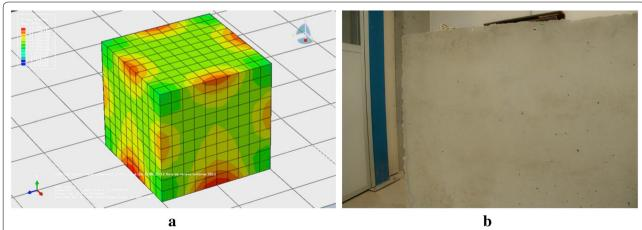
Fig. 12 a Maximum principal stress distribution (MPa) within the concrete cube 12 h after the casting; and **b** state of the cube 28 days after the curing process with no evidences of early age cracking.
