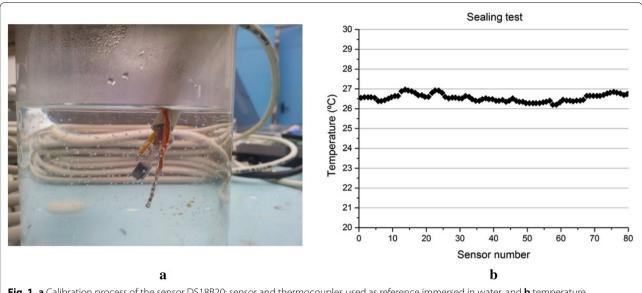
Fig. 1 a Calibration process of the sensor DS18B20: sensor and thermocouples used as reference immersed in water, and **b** temperature measurement during the sealing tests.
