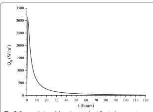
**Fig. 8** Time evolution of the volumetric heat flux in the concrete considering the hydration of the cement.
