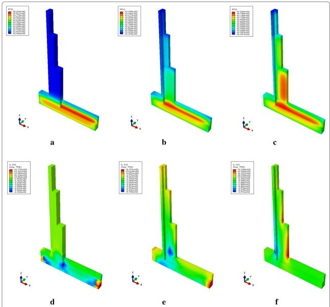
**Fig. 18** Thermo-mechanical response of the retaining wall: Temperature distribution (in  $^{\circ}$ C) at **a** 3 days; **b** 11 days; and **c** 28 days; and vertical stresses (in N/cm<sup>2</sup>) at **d** 3 days; **e** 11 days; and **f** 28 days.
