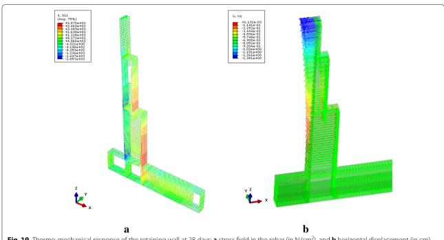
Fig. 19 Thermo-mechanical response of the retaining wall at 28 days: a stress field in the rebar (in N/cm²), and b horizontal displacement (in cm).
