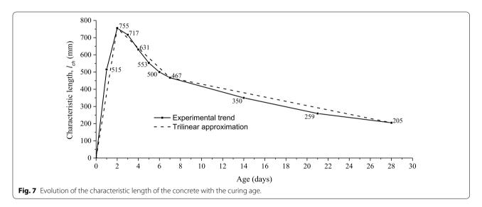
(or ductility) of concrete, it is observed that concrete exhibits a more brittle behavior with age (Cifuentes et al. 2013).
