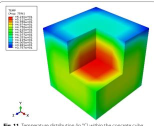
**Fig. 11** Temperature distribution (in °C) within the concrete cube 12 h after casting.
