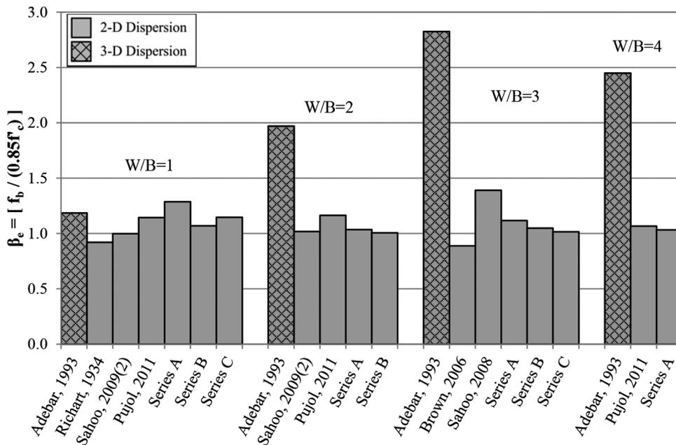
Fig. 7—Mean experimental efficiency factors across various studies for selected  $W/B$ .
