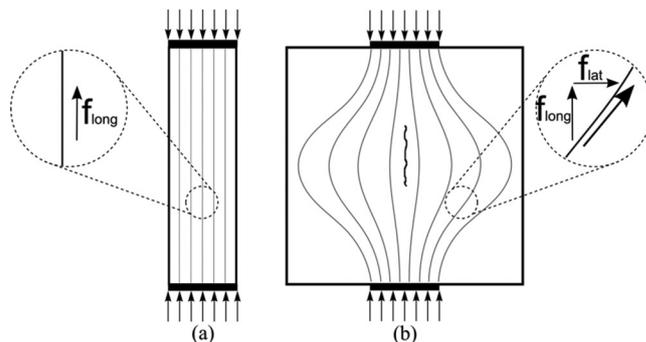
Fig. 2—Internal stresses in: (a) prismatic strut; and (b) bottle strut showing 2-D lateral dispersion.
