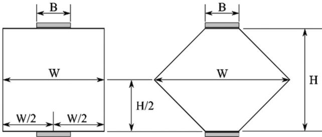
Fig. 3—Typical bottle specimen dimensions. (Note:  $B$  is out-of-plane dimension.)
