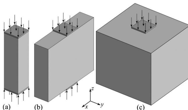
Fig. 1—Examples of: (a) rectangular prismatic strut; (b) 2-D rectangular bottle strut; and (c) 3-D rectangular bottle strut.
