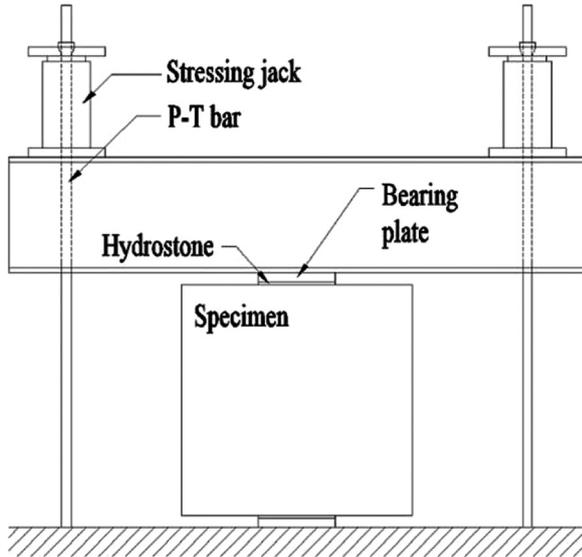
Fig. 4—Testing configuration for large specimens.
