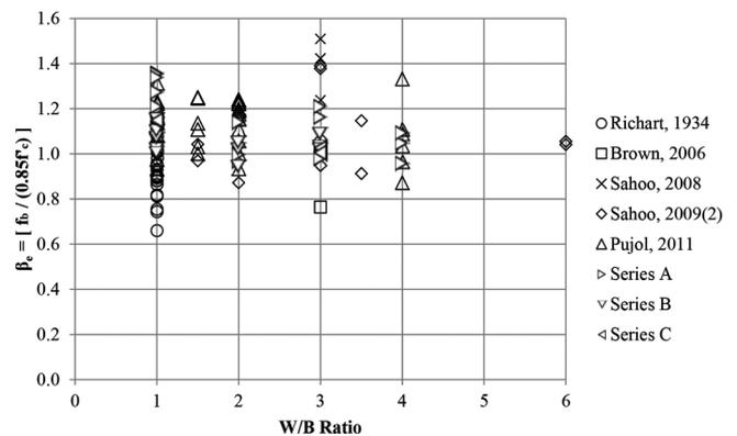
Fig. 8—Plot of experimental strut efficiency factor for 2-D dispersion and peak load.
