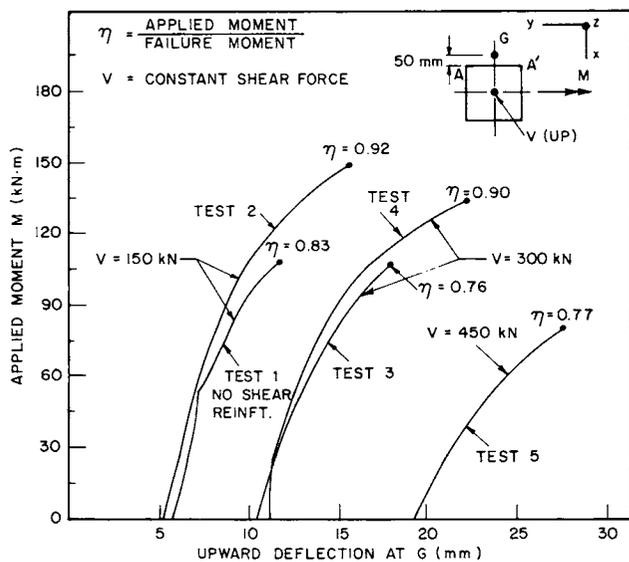
Fig. 7 — Deflection versus moment in Tests 1 to 5
