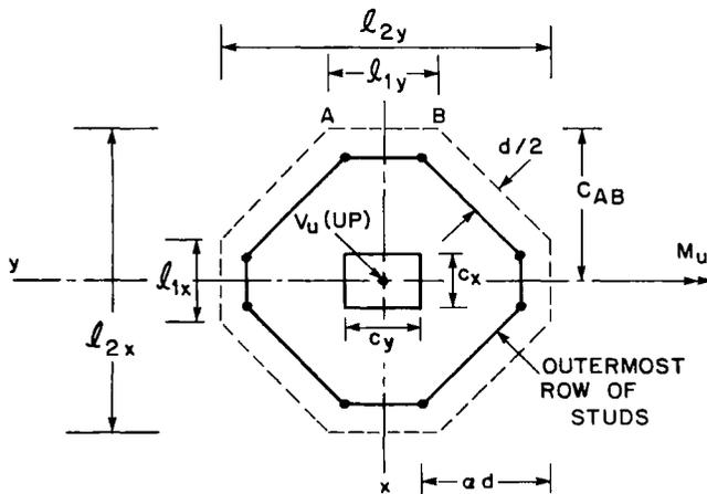
(b) AT  $d/2$  FROM THE OUTERMOST ROW OF SHEAR STUDS
