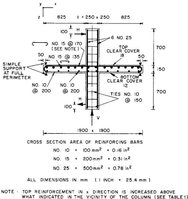
Fig. 1 — Test specimen
