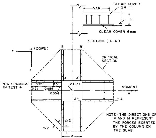
Fig. 2 — Typical stud-shear reinforcement arrangement
