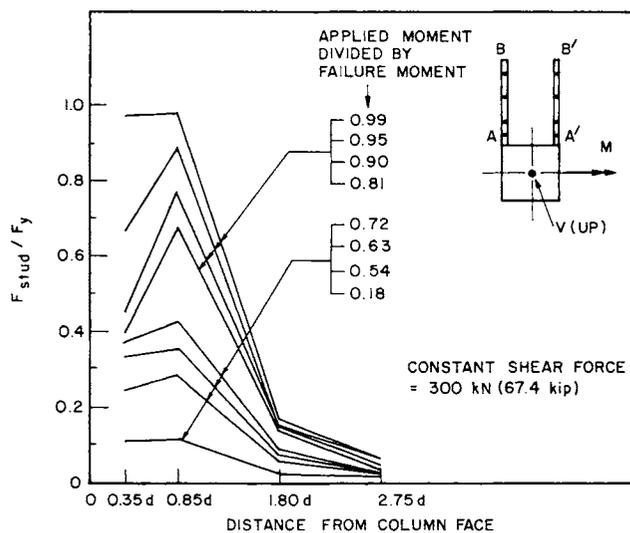
Fig. 5 — Force in studs situated on Line A'B' of Test 4
