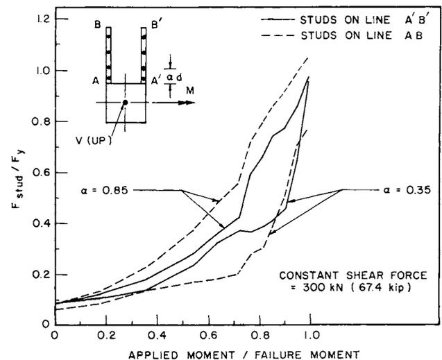
Fig. 6 — Force in studs versus applied moment on Lines AB and A'B' of Test 4
