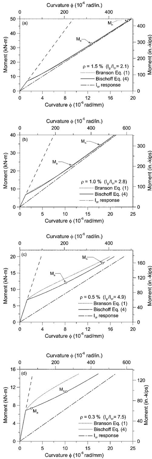
Fig. 3—Computed moment curvature response for: (a)  $\rho = 1.5\%$ ; (b)  $\rho = 1.0\%$ ; (c)  $\rho = 0.5\%$ ; and (d)  $\rho = 0.3\%$ .
