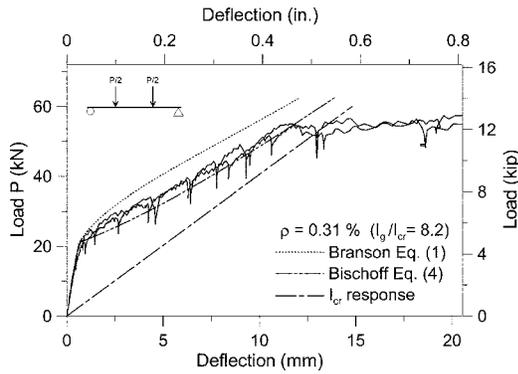
Fig. 6—Steel reinforcement beam response for  $\rho = 0.31\%$  ( $I_g/I_{cr} = 8.2$ ).
