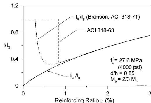
Fig. 1—Effective moment of inertia at service loads ( $M_a = 2/3M_n$ ).
