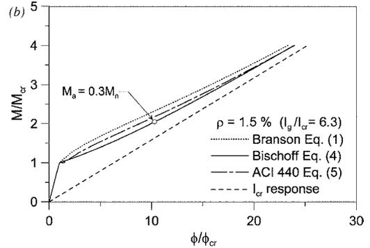
Fig. 7—GFRP beam response for: (a)  $\rho = 0.5\%$  ( $I_g/I_{cr} = 16.8$ ); and (b)  $\rho = 1.5\%$  ( $I_g/I_{cr} = 6.3$ ).
