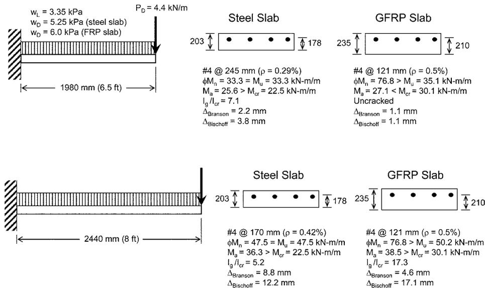
Fig. 10—Cantilever slab design examples. (Note: 1 mm = 0.04 in.; 1 m = 3.28 ft, 1 kN-m/m = 224.8 in.-lb/in., 1 kPa = 20.89 psf, and 1 kN/m = 68.5 plf).
