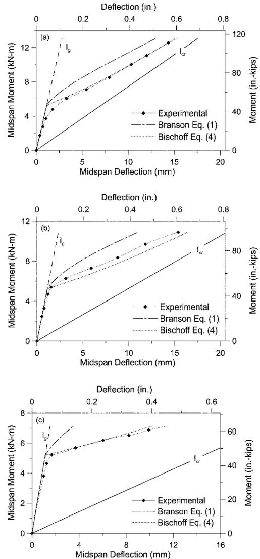
Fig. 5—Slab response for: (a)  $\rho = 0.52\%$  and  $I_g/I_{cr} = 6.3$ ; (b)  $\rho = 0.33\%$  and  $I_g/I_{cr} = 8.8$ ; and (c)  $\rho = 0.20\%$  and  $I_g/I_{cr} = 13.0$  (after Gilbert 2006).
