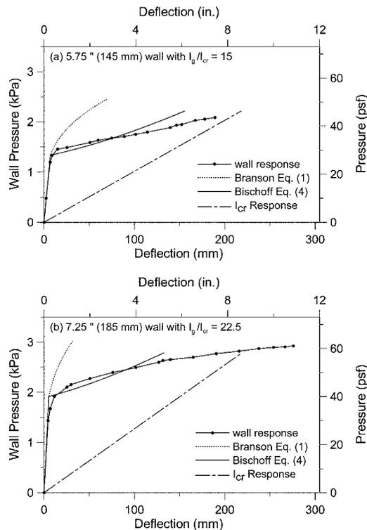
Fig. 9—Response for: (a) 145 mm (5.75 in.) thick wall ( $\rho_g = 0.28\%$ ); and (b) 185 mm (7.25 in.) thick wall ( $\rho_g = 0.23\%$ ).
