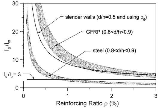
Fig. 4—Variation of  $I_g/I_{cr}$  ratio with reinforcing ratio.
