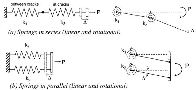
Fig. 2—Simple spring models.
