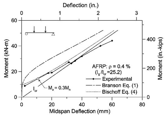
Fig. 8—AFRP beam response comparison ( $I_g/I_{cr} = 25.2$ ).
