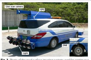
Fig. 3 Photo of the road surface imaging system used for continuous surface image acquisition on the pilot bridge.
