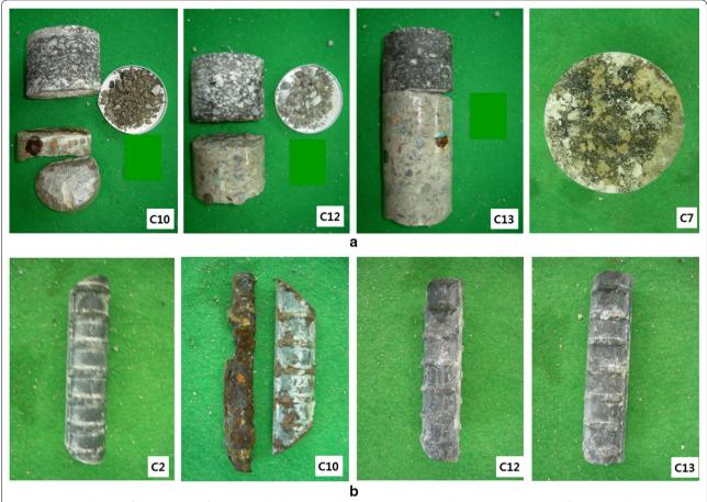
Fig. 5 Visual evaluation of deterioration of concrete and rebar through core samples; a major deterioration pattern and b rebar condition.
