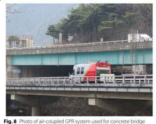
**Fig. 8** Photo of air-coupled GPR system used for concrete bridge deck survey in this study.
