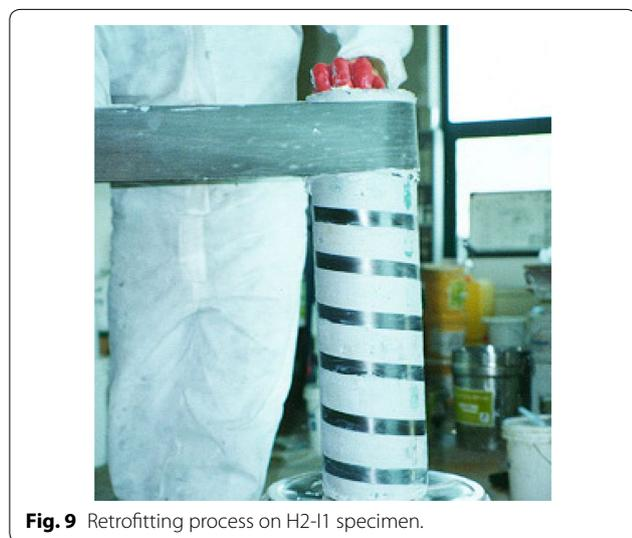
**Fig. 9** Retrofitting process on H2-I1 specimen.
