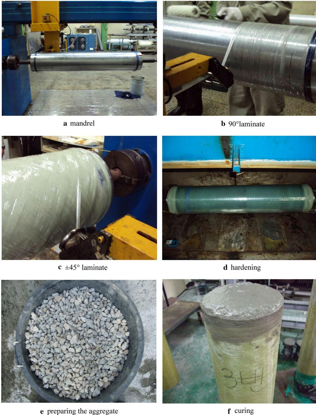
**Fig. 1** Fabrication process for testing.
