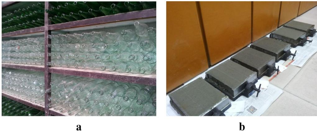
**Fig. 1** Cement mortar incorporating waste glass powder for alkali-silica reaction expansion test. **a** Waste glass, **b** specimen after casting.
