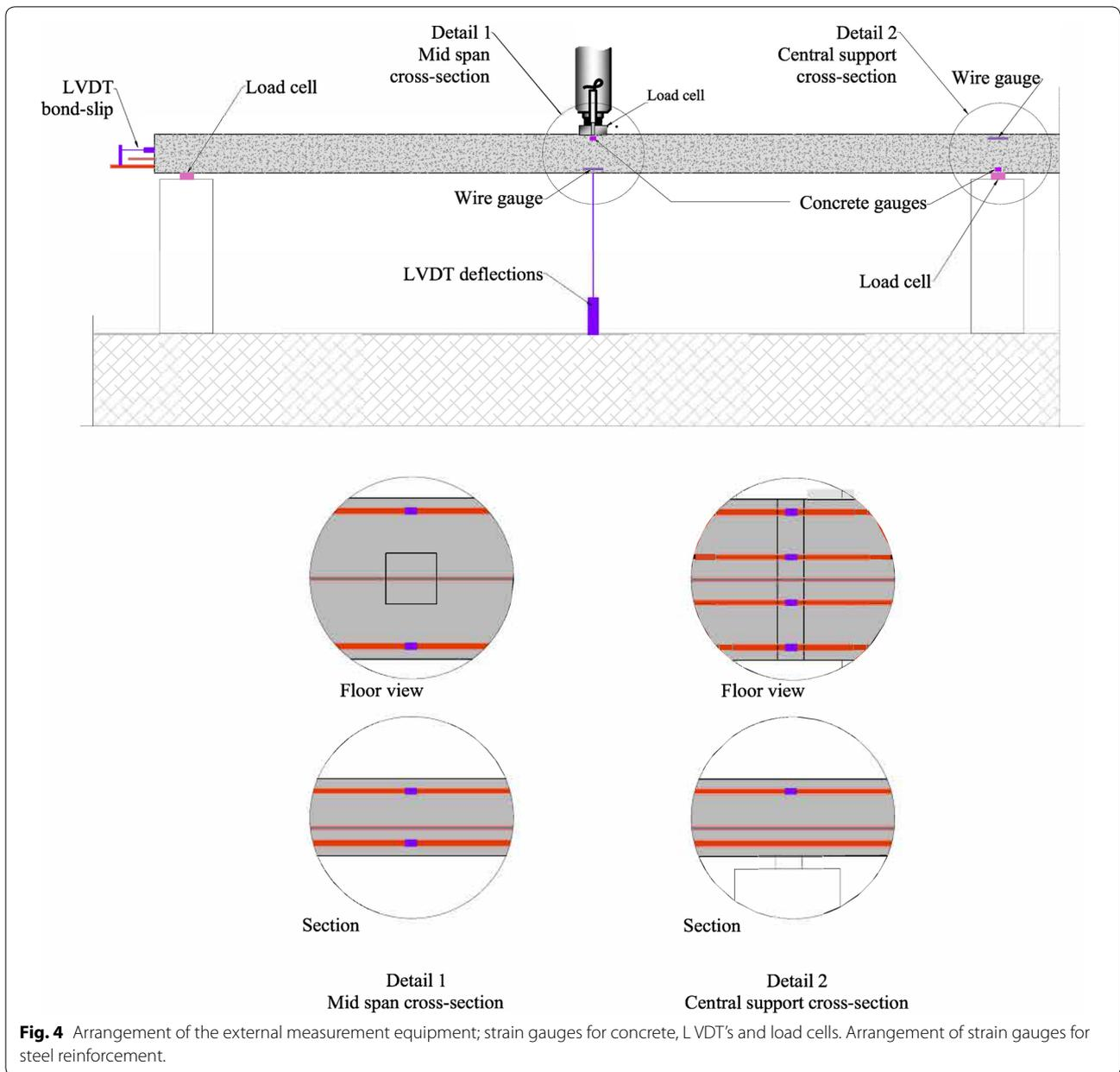
**Fig. 4** Arrangement of the external measurement equipment; strain gauges for concrete, LVDT's and load cells. Arrangement of strain gauges for steel reinforcement.
