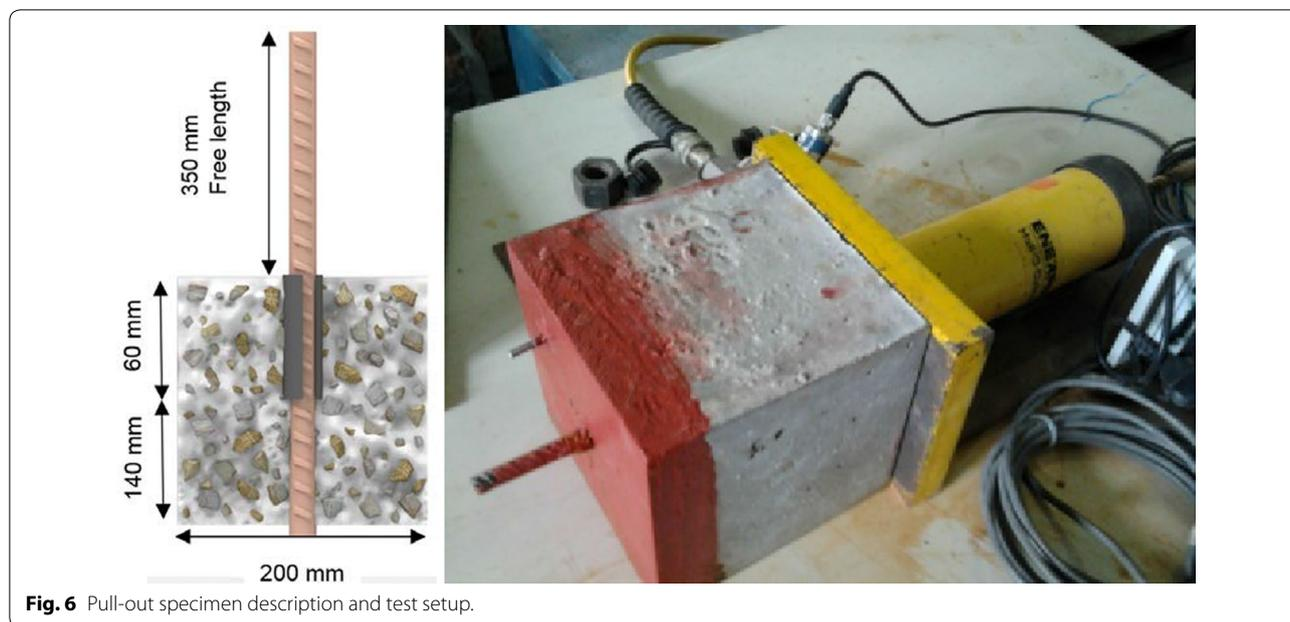
**Fig. 6** Pull-out specimen description and test setup.
