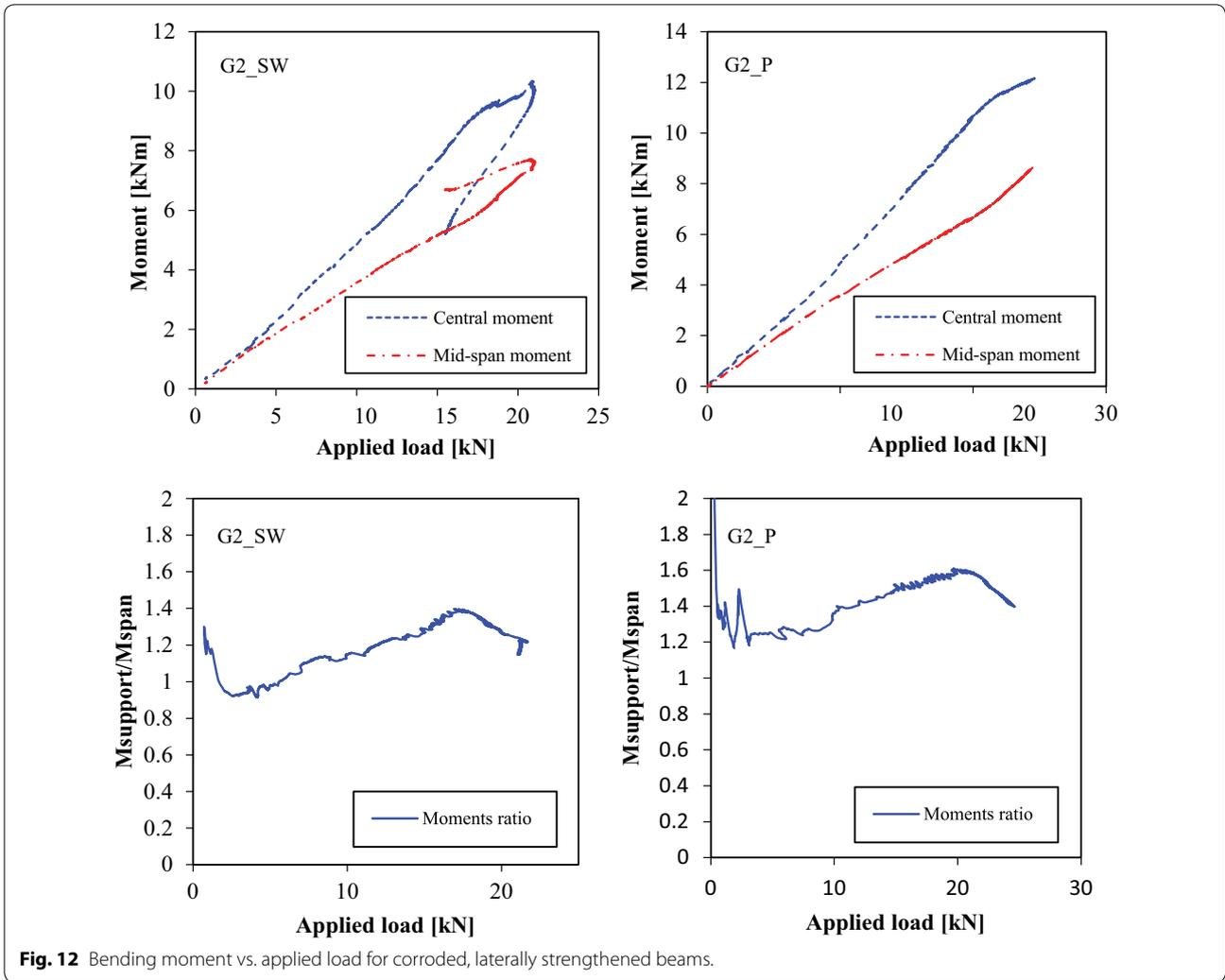
**Fig. 12** Bending moment vs. applied load for corroded, laterally strengthened beams.
