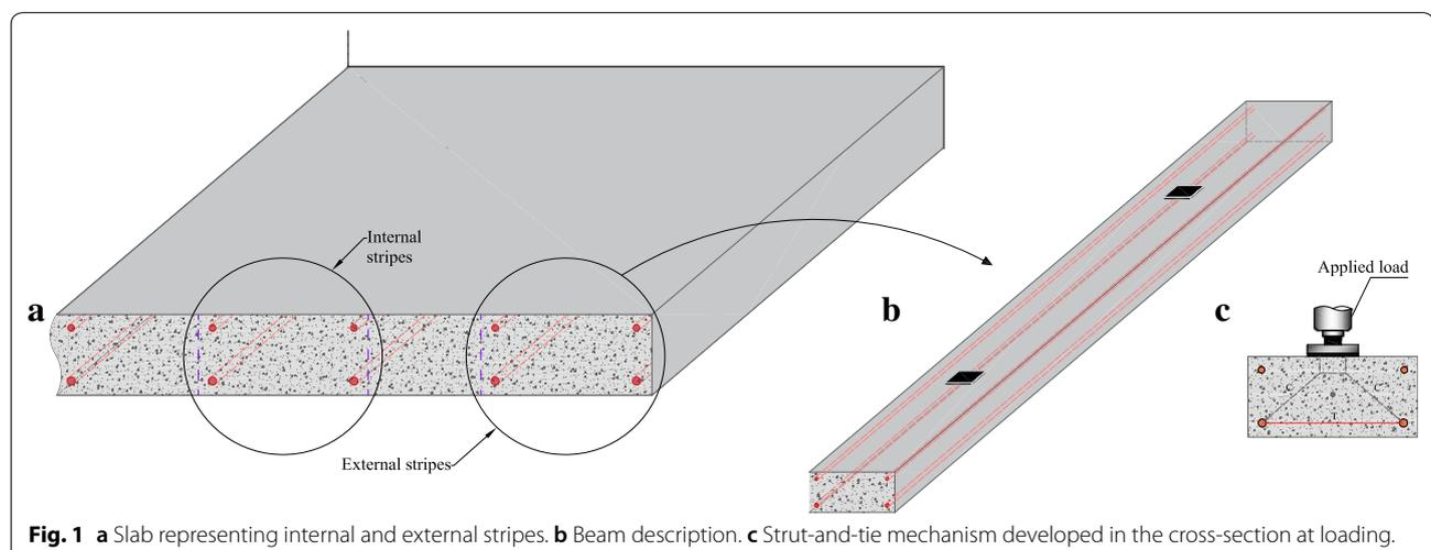
**Fig. 1** a Slab representing internal and external stripes. b Beam description. c Strut-and-tie mechanism developed in the cross-section at loading.
