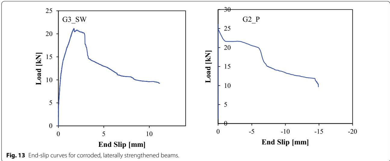
**Fig. 13** End-slip curves for corroded, laterally strengthened beams.
