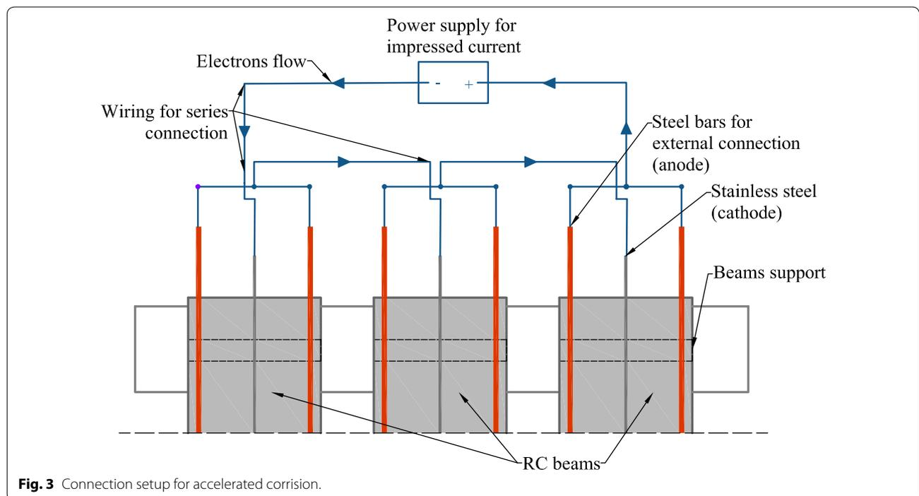
**Fig. 3** Connection setup for accelerated corrosion.
