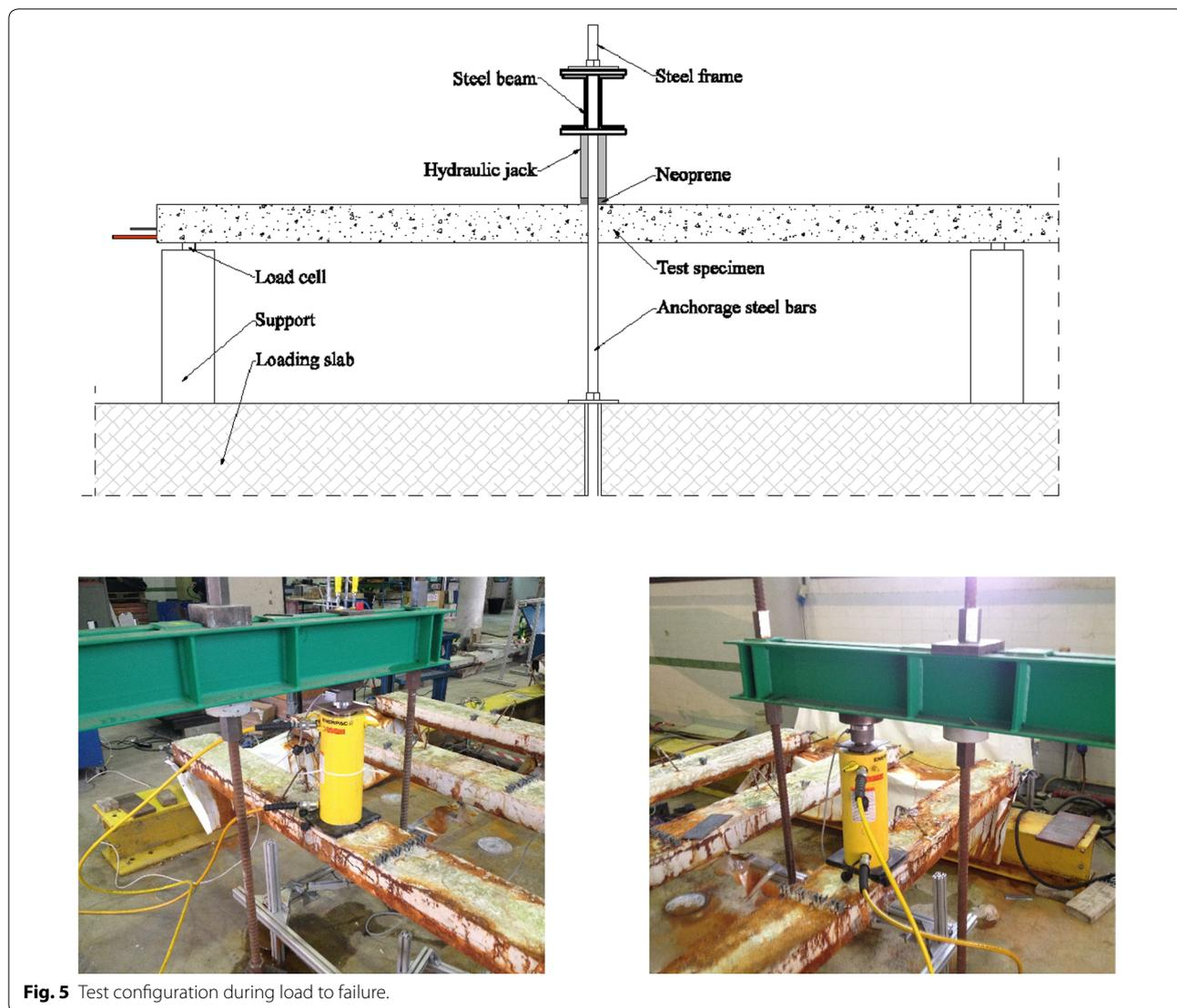
**Fig. 5** Test configuration during load to failure.
