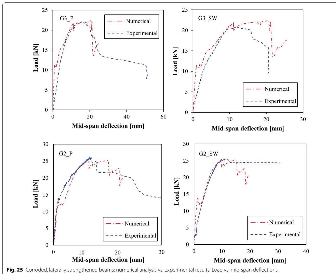
**Fig. 25** Corroded, laterally strengthened beams: numerical analysis vs. experimental results. Load vs. mid-span deflections.
