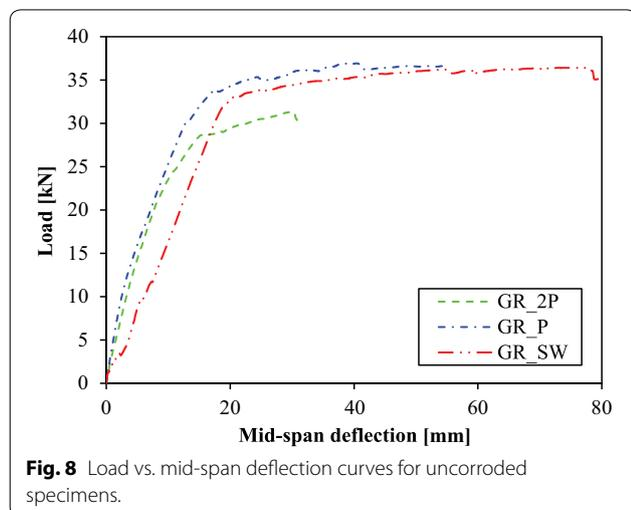
**Fig. 8** Load vs. mid-span deflection curves for uncorroded specimens.
