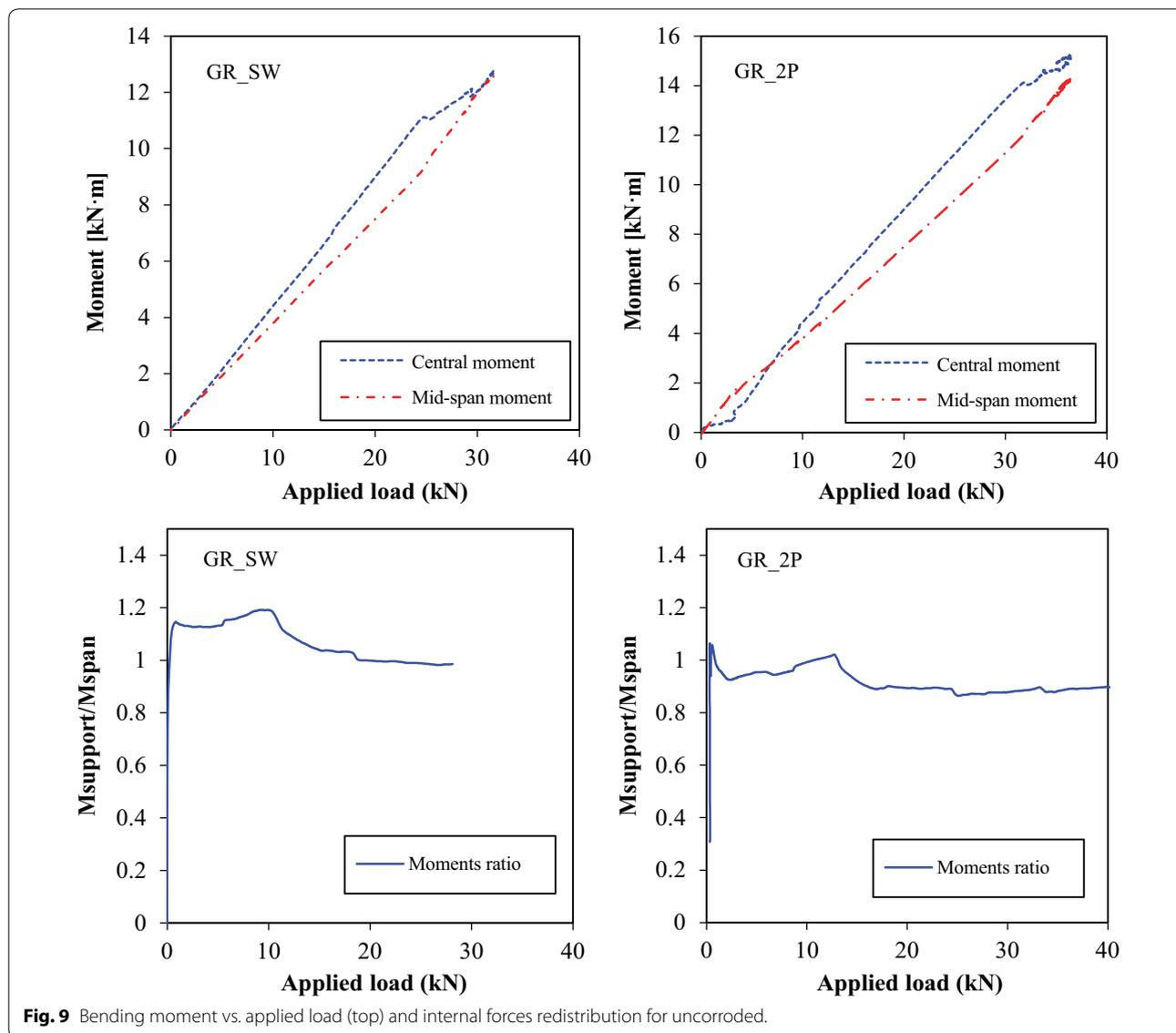
**Fig. 9** Bending moment vs. applied load (top) and internal forces redistribution for uncorroded.
