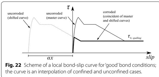
**Fig. 22** Scheme of a local bond-slip curve for 'good' bond conditions; the curve is an interpolation of confined and unconfined cases.
