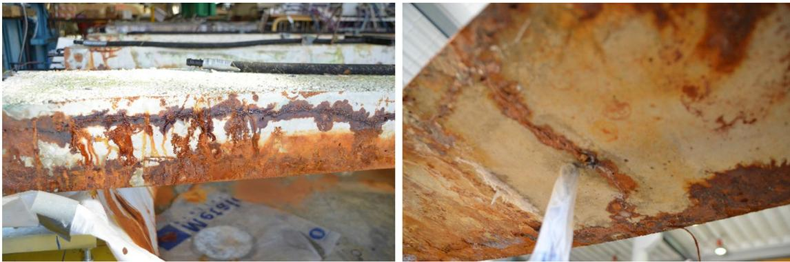
**Fig. 7** Deterioration at the end of the accelerated corrosion process: (left) longitudinal and (right) transverse cracks.
